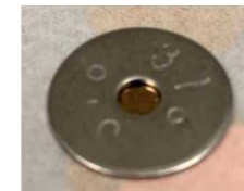
Washer No 6, 0.625 in diameter 0.6-0.96 mm thick 3.8 mm opening in washer Ag epoxy to connect washer
