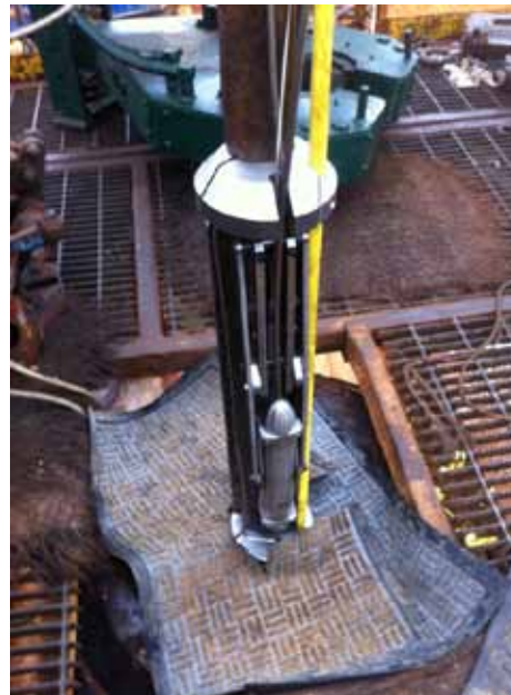
Geophone pod and clamp assembly
