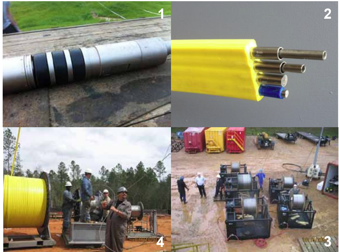
1. Hydroset packer; 2. flat pack and control lines; 3. old deployment method with multiple spools; 4. newer, cleaner deployment with flat pack
