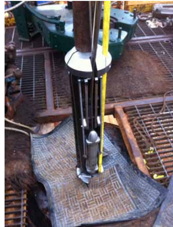
Geophone pod and clamping assembly
