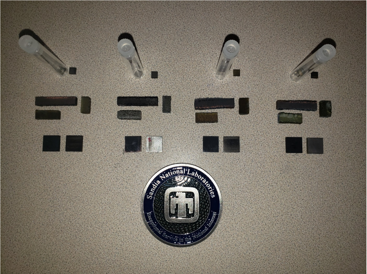
Figure 1-4. RLEA and RHEA test samples printed at SNL during 2020 using the LENS approach.
