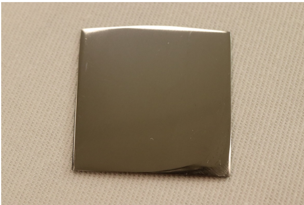
Figure 2-4. Polished HfNbTaZr RHEA sample.
