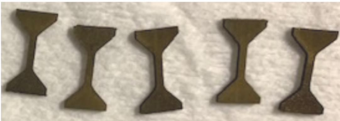
Figure 1-5. NbTaVW RHEA Type A dogbone specimens printed via the LENS machine.
