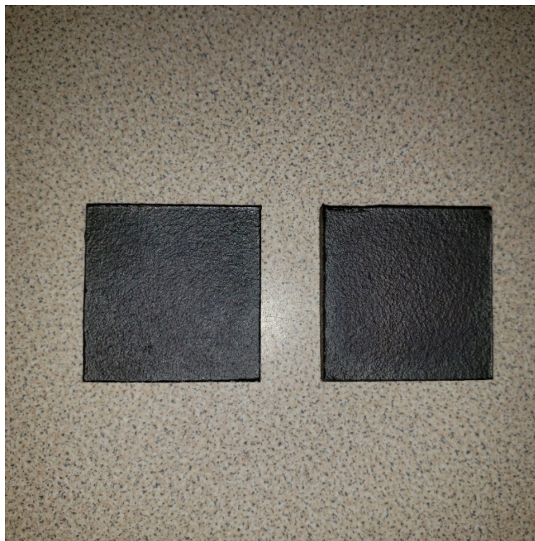
Figure 3-2. HfNbTaZr SPS 1-inch rectangular cuboids.
