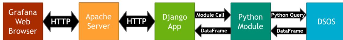
Figure 3-7 Analysis and Visualization Pipeline Block Diagram . Queries from a Grafana web browser are sent through an Apache server to a Django application. The queries can specify a Python analysis module to call, which queries the DSOS database and manipulates the returned DataFrame . This DataFrame is returned to the Grafana browser after being correctly formatted to create meaningful visualizations.
