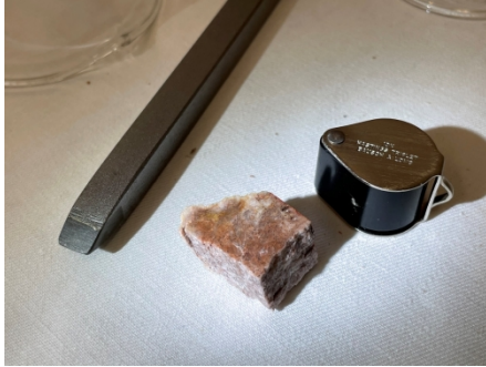
Figure 1: microcline rock from which samples were mechanically cleaved
