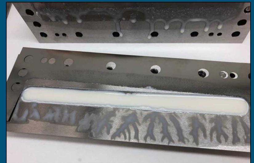
Print failure due to clogged slot die
