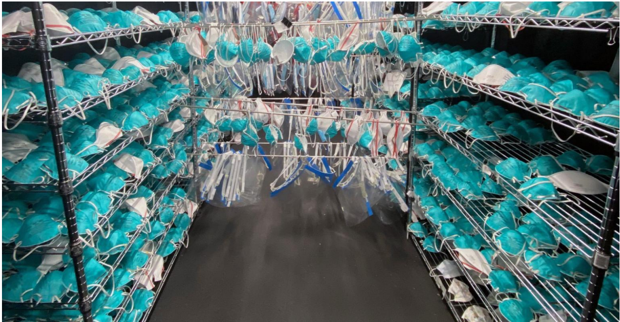
Figure 4: 3M 1860 masks being racked for Batelle’s hydrogen peroxide vapor sterilization process.
