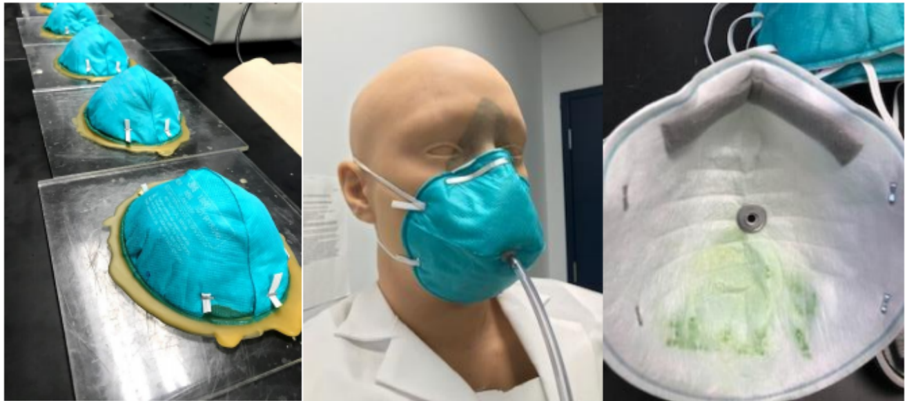
Figure 20: Left-hand panel: SC-CO 2 treated masks affixed to planar flange for flow resistance measurements. Center panel: SC-CO 2 treated masks tested for proper fit under standardized pressure/flow conditions. Right-hand panel: Discoloration resulting from transfer of dye from an adjacent mask during immersion in SC-CO 2 . The use of a SC-CO 2 colorfast dye would be desirable to prevent such staining, because aesthetics has a bearing on the willingness of health care workers to reuse masks.
