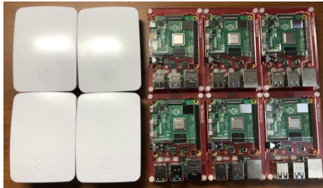
Figure 19: Raspberry Pi 3B+ and 4B computers configured with DER Simulator software.
