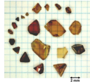
c-BN crystals produced at high pressure. Taniguchi, Comprehensive Hard Materials , 3, 587 (2014).
