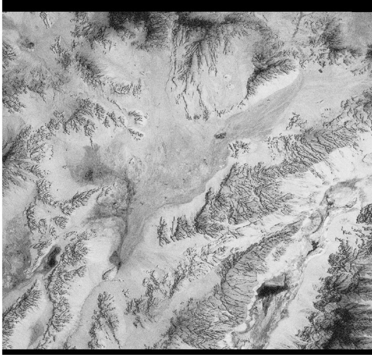
Figure 2-3: Coherence of images 4 and 5 in radar coordinates. Near range is the right edge of the image. Far range is the left edge of the image. Cross range is up and down. White is high coherence. Black is low coherence or no data. Shadows and water have low coherence.
