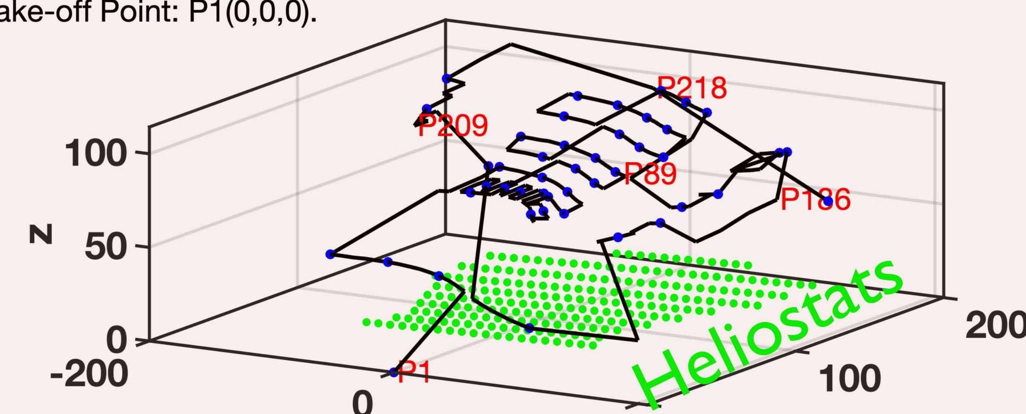
For demonstration purposes 45 flight path points that correspond to 45 heliostats (out of 218 heliostats at NSTTF) are depicted.
