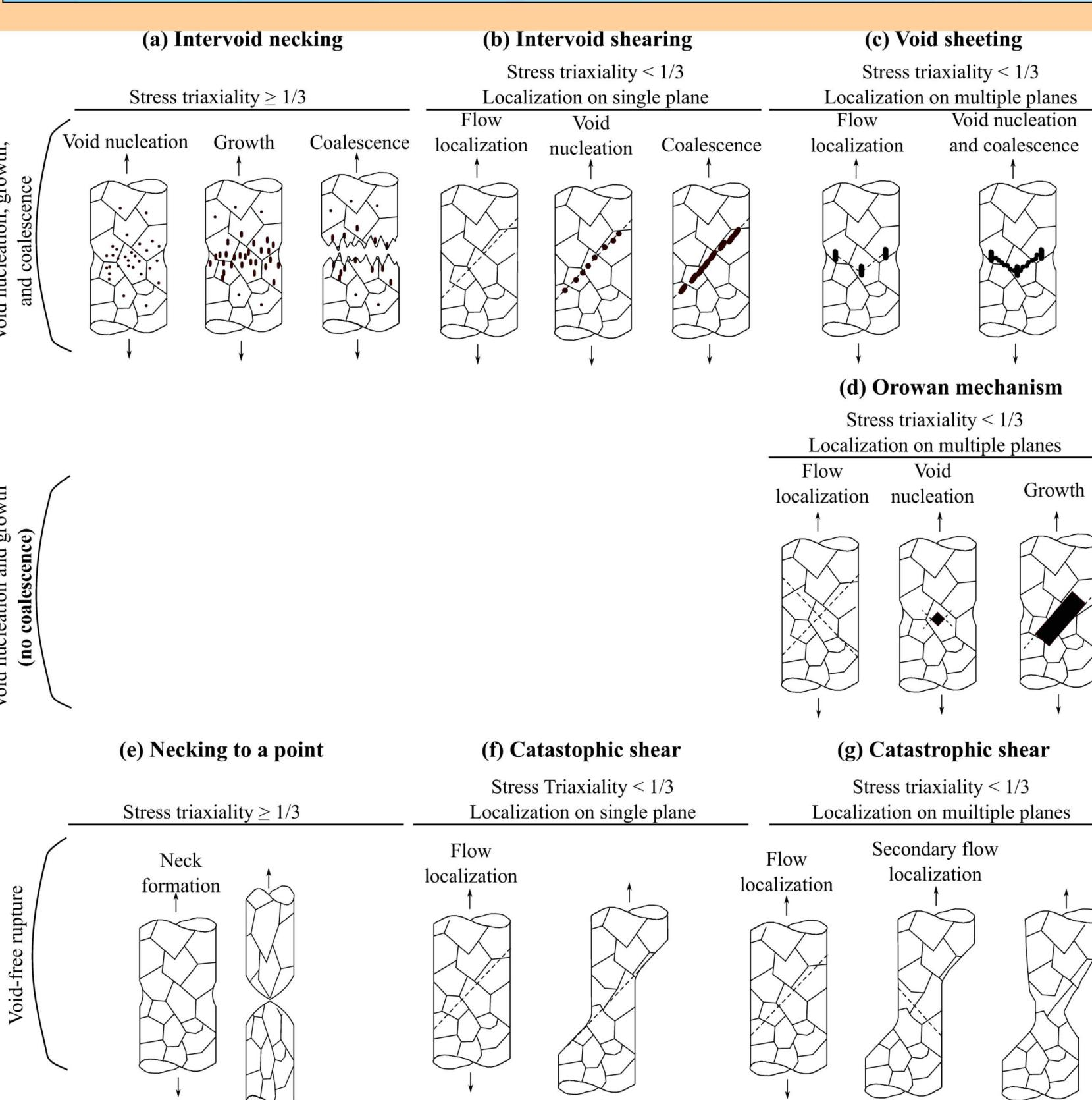
At least seven different failure mechanisms have been observed in different materials. However, all but intervoid necking and intervoid shearing have largely been ignored. Thus, there is no understanding of:
