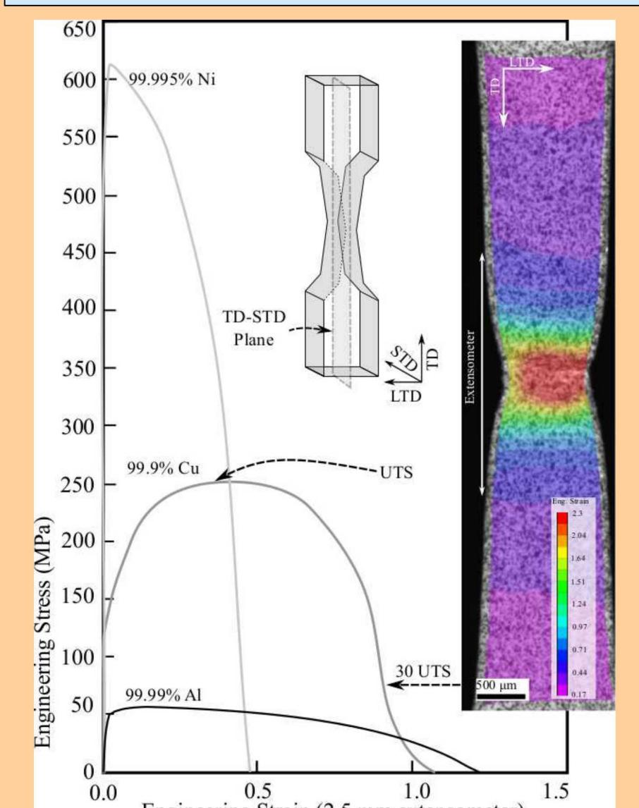
The fracture process was examined in high-purity aluminum (Al), copper (Cu), and nickel (Ni). Damage accumulation was characterized by interrupting tensile tests of different specimens of each material at predetermined percentages of the UTS. Specimens were subsequently ground and polished to the midplane to characterize the progression of damage
