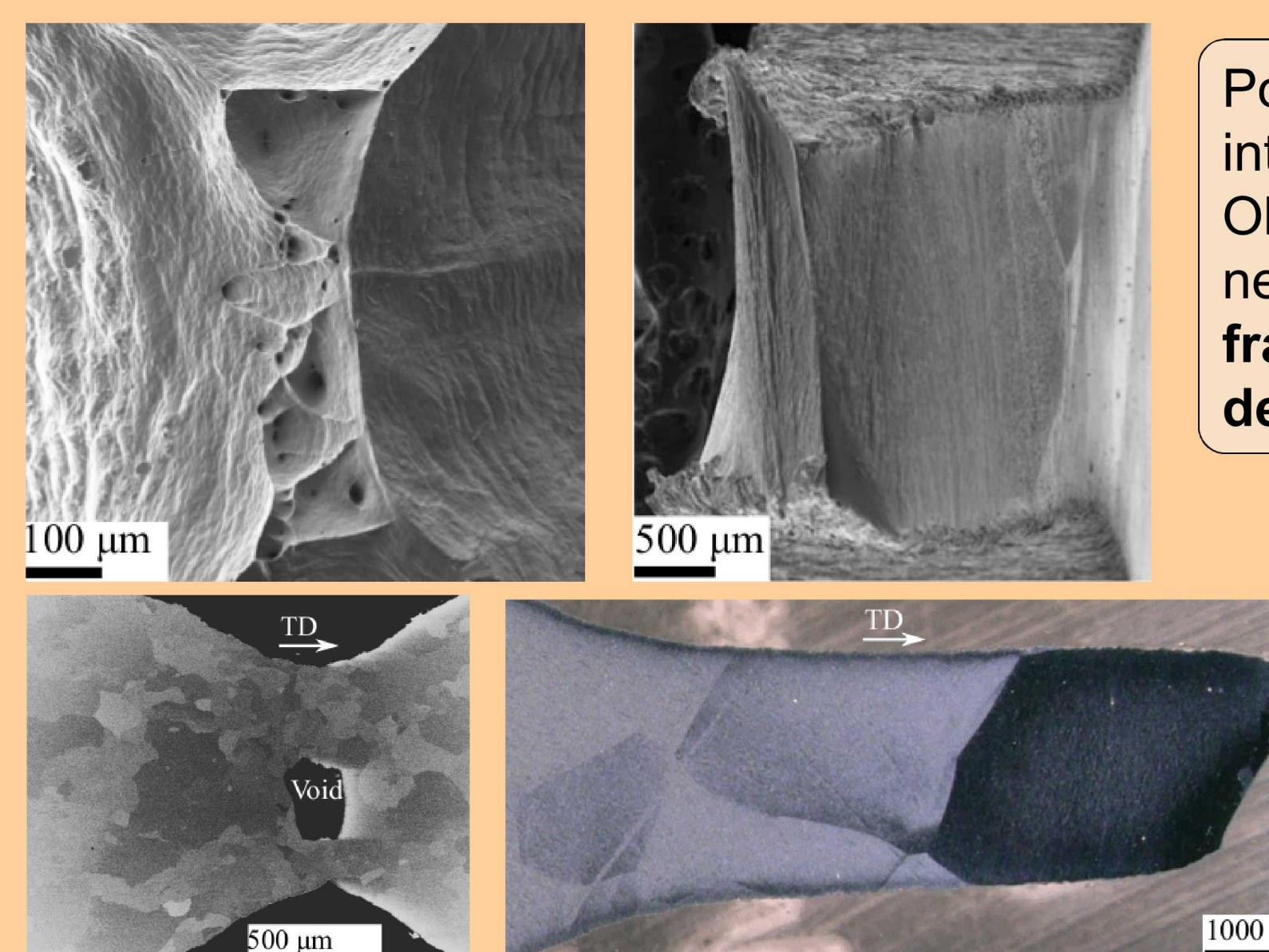
Polycrystalline Al failed by intervoid necking while Oligocrystalline Al failed by necking of a point. The fracture mechanism in Al depended on grain size.
