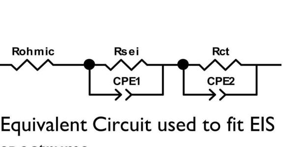
Equivalent Circuit used to fit EIS spectra
