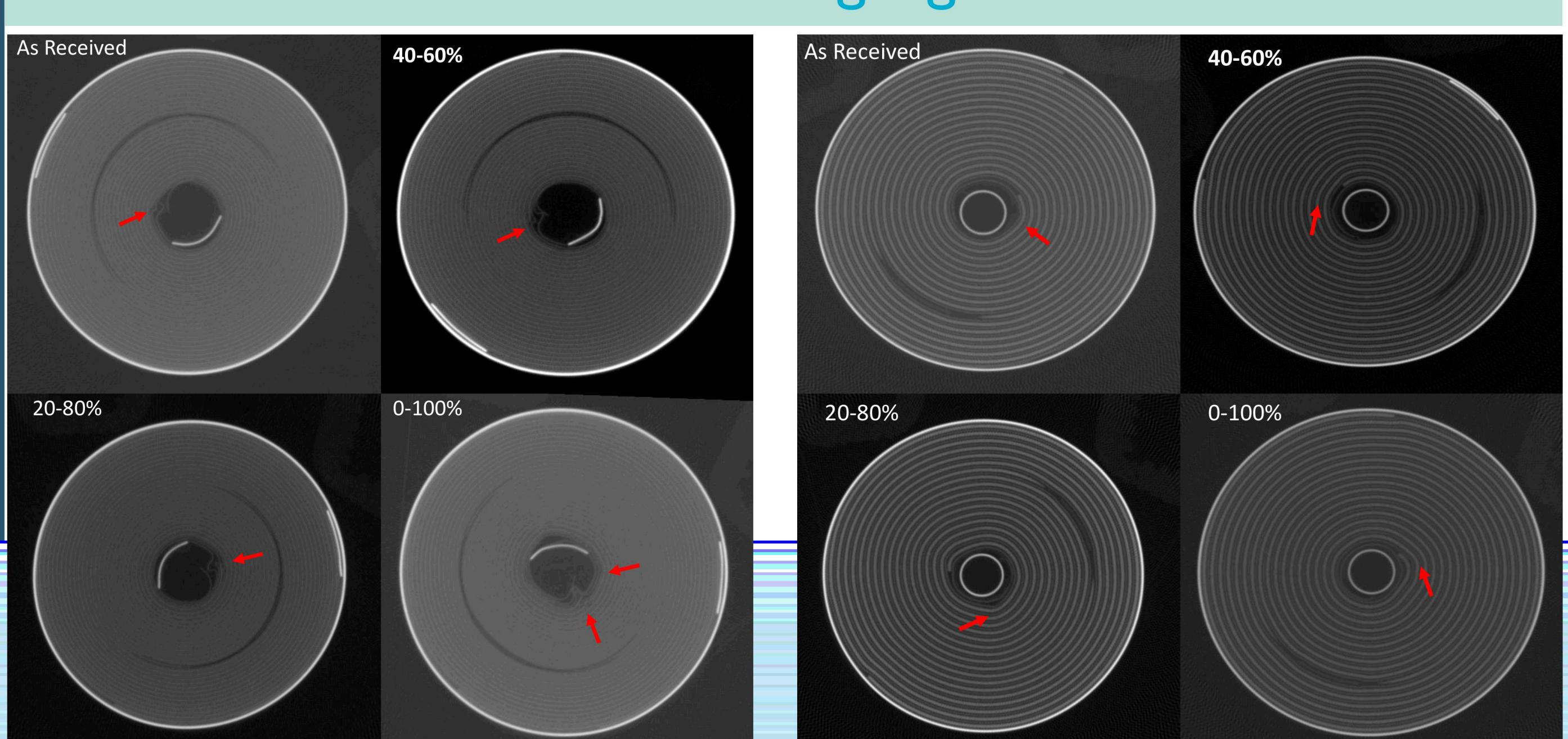
Mid-section CT Scan of NMC (Left) and NCA (Right) cells at 0% SOC (by voltage) as received and cycled to 80% capacity in listed SOC range at 0.5C and at 25C
