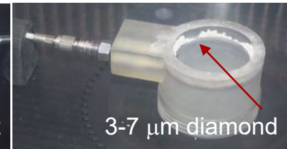
Particulates can be loaded in Al shock tube, or PMMA nozzles (below)
