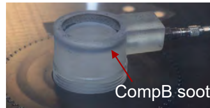
Particulates can be loaded in Al shock tube, or PMMA nozzles (below)
