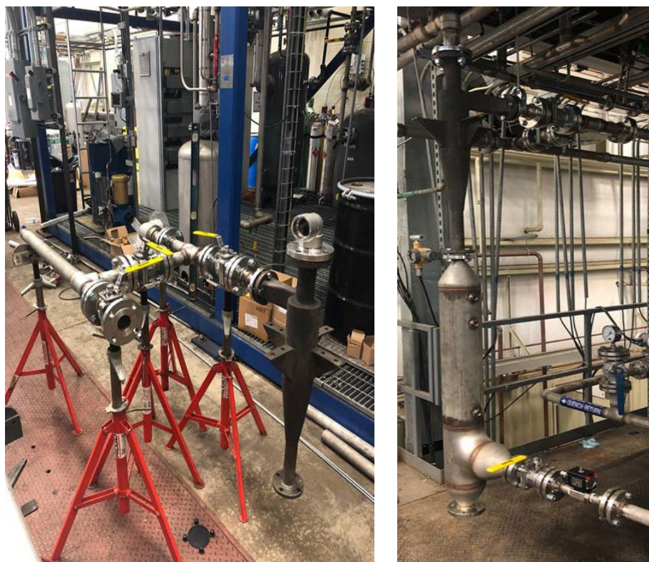
Exhibit 24. Cyclone separator and bypass welding setup (left) and cyclone separator installed with sump level control (right).
