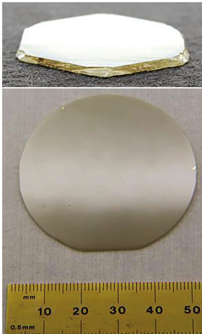
Figure 7: 2 inch GaN crystal and wafer fabricated by Soraa's process (from ref 44)
