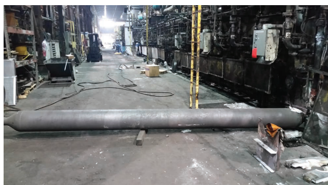
Figure 2: Furnace roll made with the ORNL team's alloy. This roll appears pristine after being in a plate austenitizing furnace at 900°C for 4000 hours. Compared to state-of-the-art alloy furnace rolls, the new rolls result in significantly lower maintenance costs and improved productivity.
