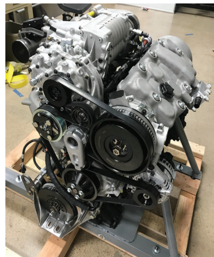
Figure 1: three-cylinder OP-GCI engine.
