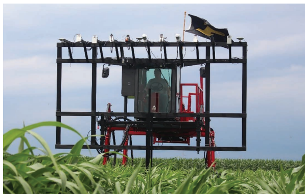
Figure 5 (left): The PhenoRover integrates visible, multispectral, ranging, and hyperspectral sensors Figure 6 (right): Automated plant identification.
