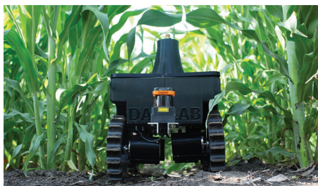
Figure 8: TerraSentia is an ultra-compact 3D-printed robot.
