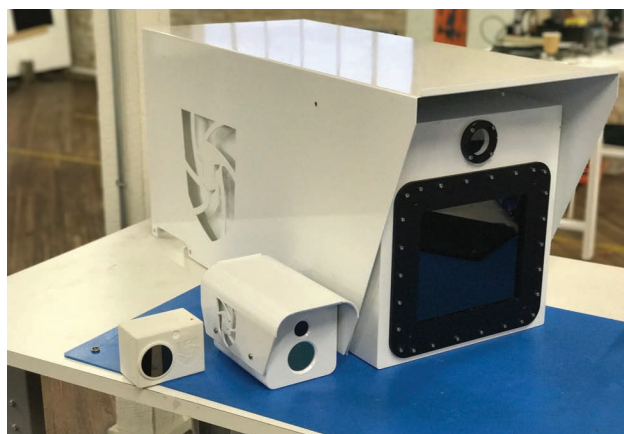
Figure 1: Under this project, Rebellion has miniaturized their gas cloud imager – the GCI (right). The mini-GCI (middle) is a mid-project functional prototype for which the team has already taken orders. The team will be shortly testing an even smaller goGCI (left) which will be 4.25in x 3.25in x 2.60in, 1 lb., battery powered, and will include embedded gas detection analytics.
