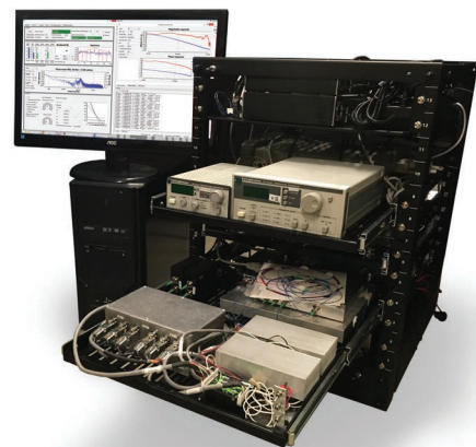
Figure 1: Under this project, the CU-Boulder team developed a solution capable of monitoring hundreds of wellpads from a central location (left). The dual-comb spectrometer has been reduced to a system that fits in a 19-inch rack mount and is robust and portable (right).
