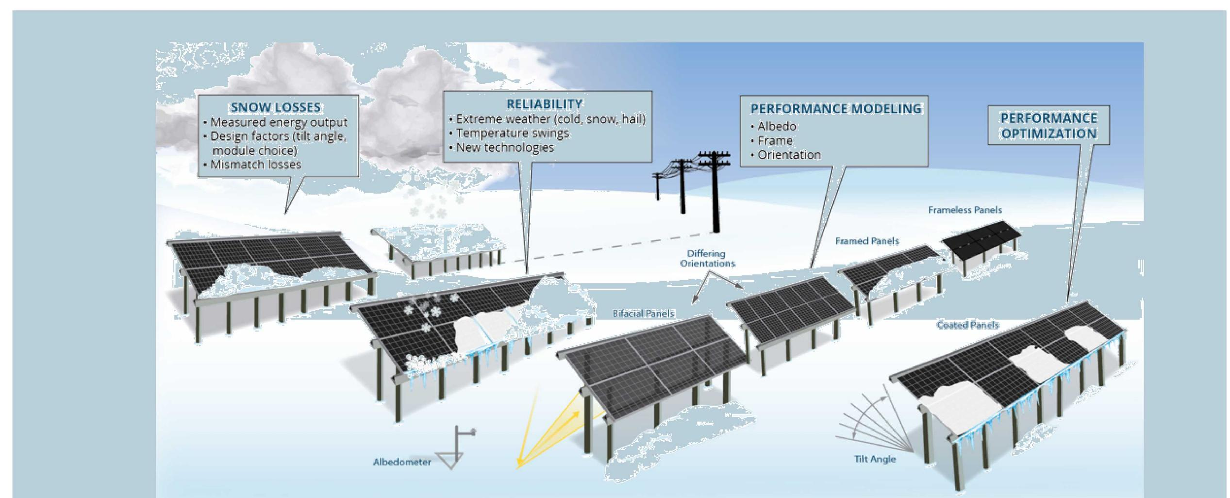
Sandia-led investigation of the impact of snow on PV system performance and reliability is focused on the multiple challenges shown in this figure.
