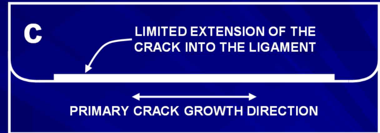
GROWTH AND COALESCENCE INTO A LONG, SHALLOW SURFACE CRACK
