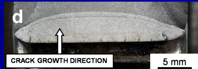
GROWTH OF THE LONG, SHALLOW SURFACE CRACK THROUGH THE LIGAMENT
