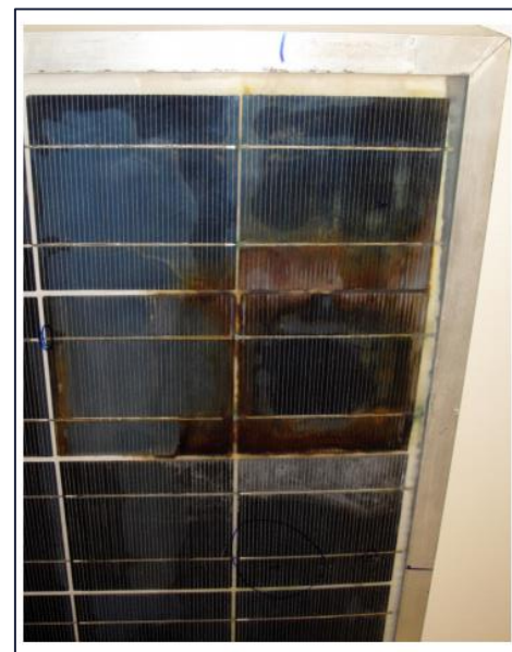
Image above: glass/glass PV module failure. Source: PVPS, Report IEA-PVPS T13-09:2017
