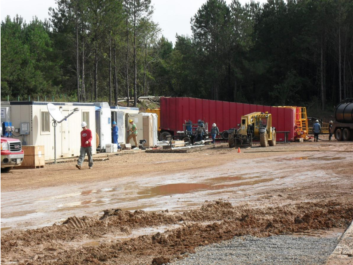
Figure 2. Office container with satellite disk dish in the foreground; U-tube portable lab designed and fabricated by LBNL in the mid-ground. Red and yellow frac tanks in the background are used for water management.
