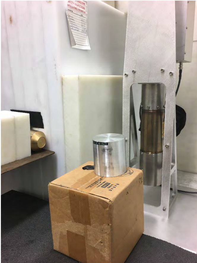
Experimental setup with Aluminum target facing STNG tube, and CLYC detector.
