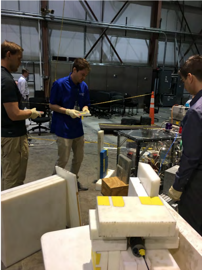
Experimental setup with CLYC detector facing DU target for DPF.
