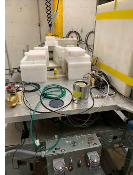
Two-detector setup with new larger elpasolite detectors on the left and on the right of the neutron source in the far background.
