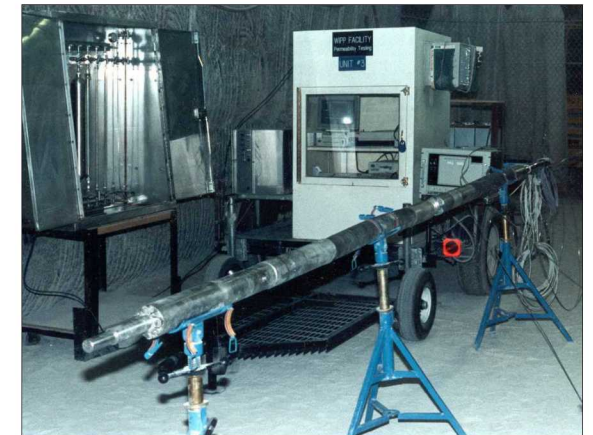
WIPP brine permeability testing
