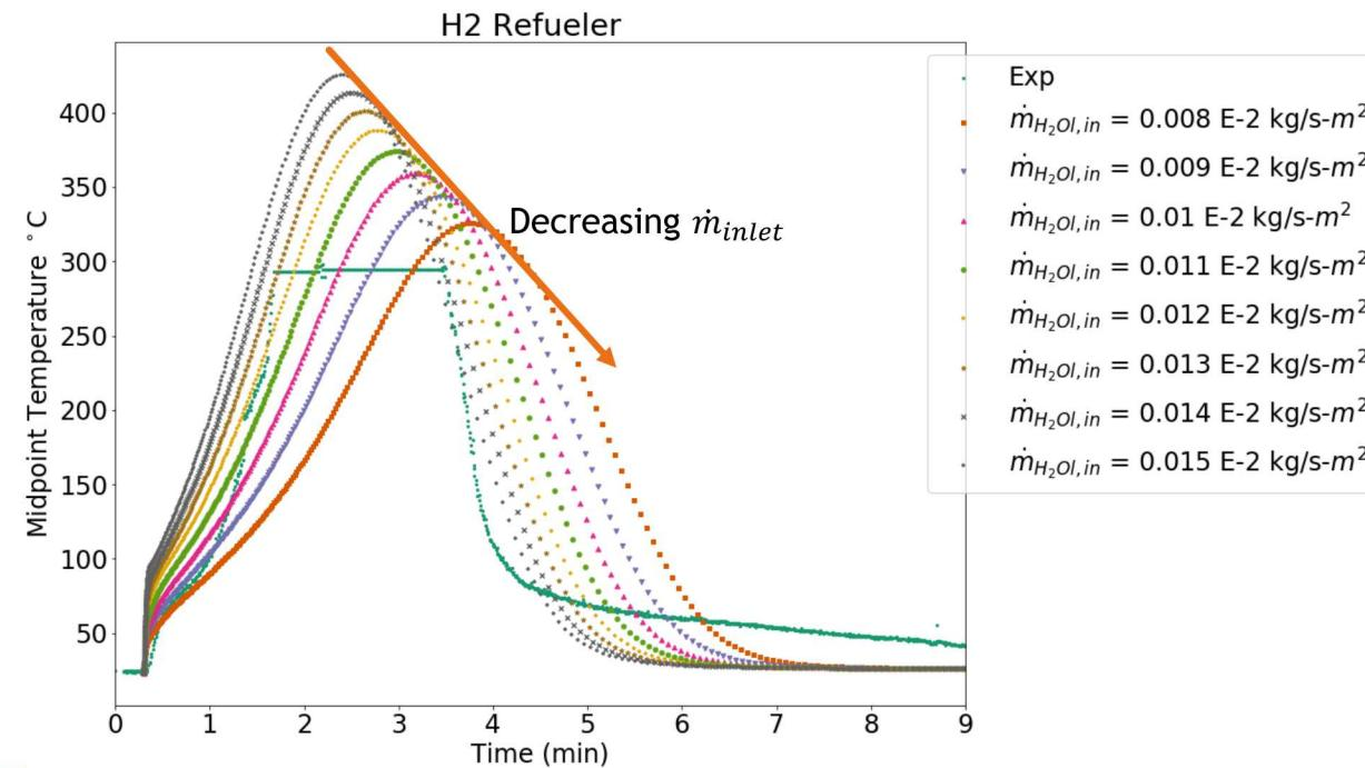
Robust numerical model demonstrates the impact of water feed to control LiH temperature and predicts that the amount of water flux directly governs the overall H<sub>2</sub> production.
