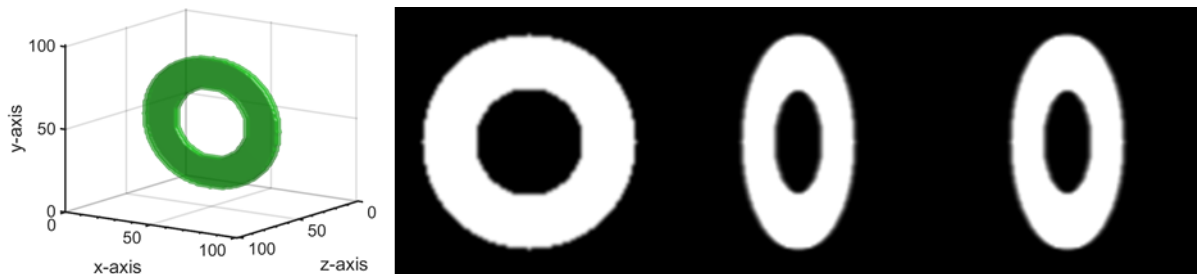
Figure 5. Isocontours of the ring volume orientation 1 (left), and linear projections at 0, 120, and 240° (right).
