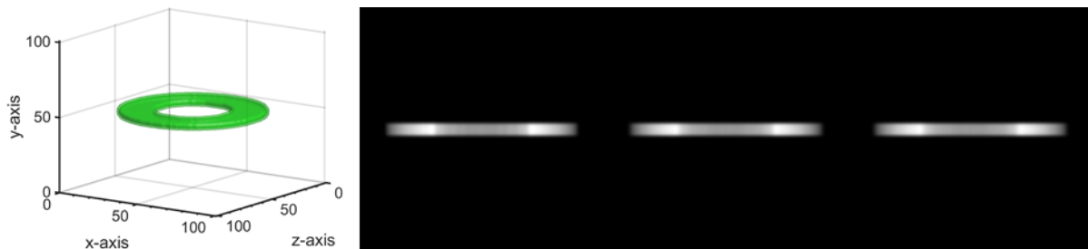
Figure 7. Isocontours of the ring volume orientation 2 (left), and linear projections at 0, 120, and 240° (right).
