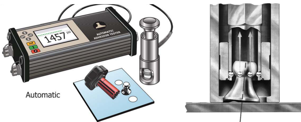
Figure 10. Automatic adhesion tester (left) and cross-sectional schematic of pull-off mechanism (right) [38].
