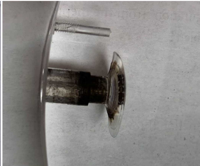
Fracture due to RP – 80 Bridgewire
