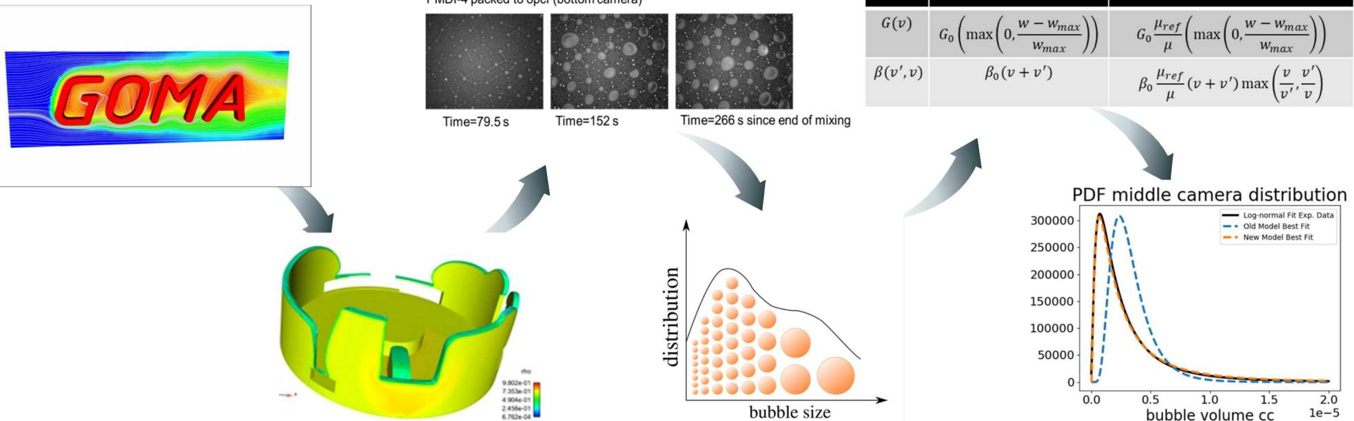
Coupled CFD-PBE for polyurethane process model and property predictions
