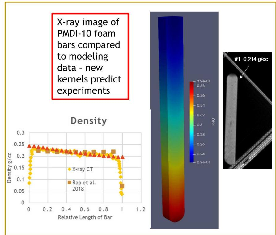
Model can now predict foam filling, curing, and bubble-size distribution for thermal conductivity
