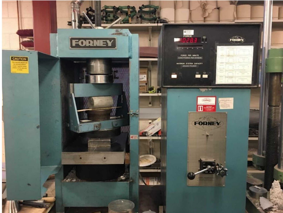
Tensile splitting (Brazilian test) equipment. Cylindrical cement sample is in load frame on left, control system is on right.
