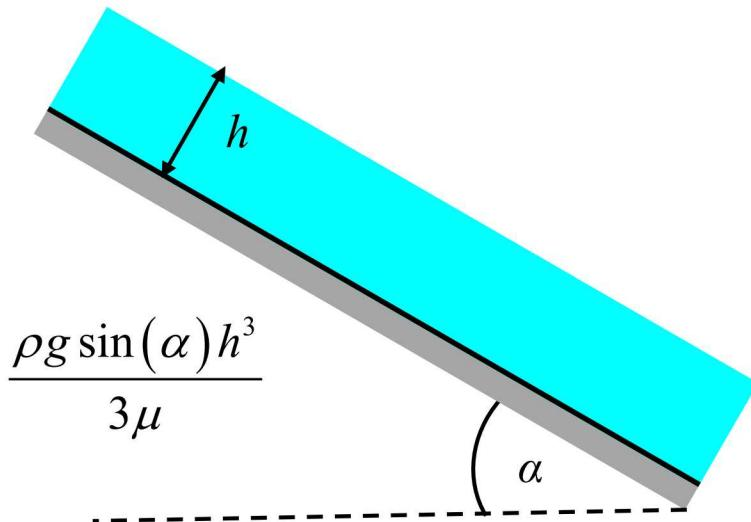
Yih, C.S. (1963) "Stability of liquid flow down an inclined plane." *The Physics of Fluids* 6(3): 321-334.
