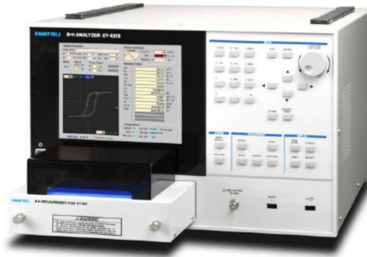
Iwatsu B-H analyzer (measurements up to 10 MHz and 150 °C)
