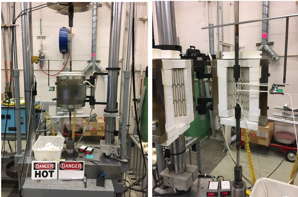
Figure 3. Three zone ATS furnace and controller (left) and specimen after failure (right).
