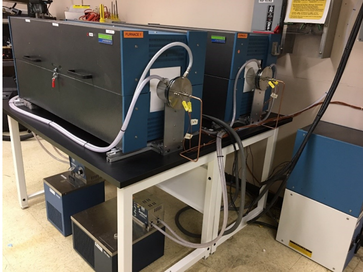
Figure 1. Tube furnace used for high temperature CO 2 corrosion tests.
