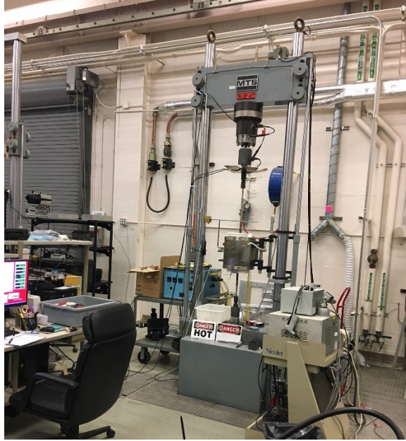
Figure 2. Elevated temperature tensile test setup on 50 kip Axial/Torsional test frame.
