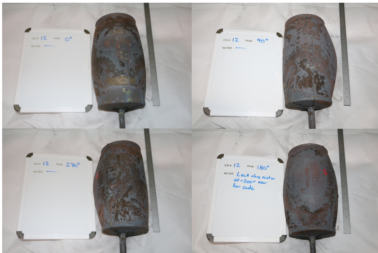
Figure 4-12. Post-test conditions of test vessel for Sequence 5. Angle positions refer to the visible portion of the vessel (see Figure 2-4). Angular positions, in clockwise direction, starting from upper left quadrant: 0°, 90°, 180°, and 270°.
