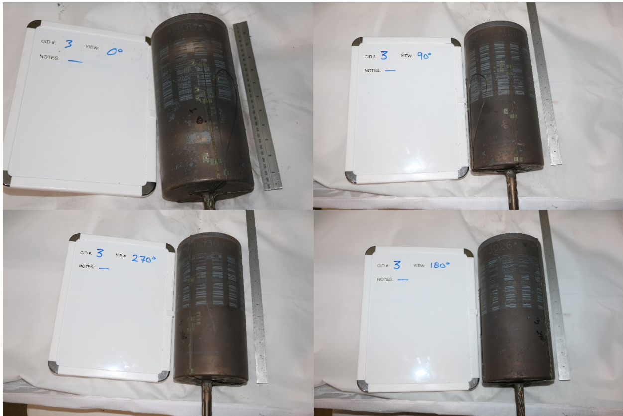
Figure 4-2. Post-test conditions of test vessel for Sequence 1. Angle positions refer to the visible portion of the vessel (see Figure 2-4). Angular positions, in clockwise direction, starting from upper left quadrant: 0°, 90°, 180°, and 270°.
