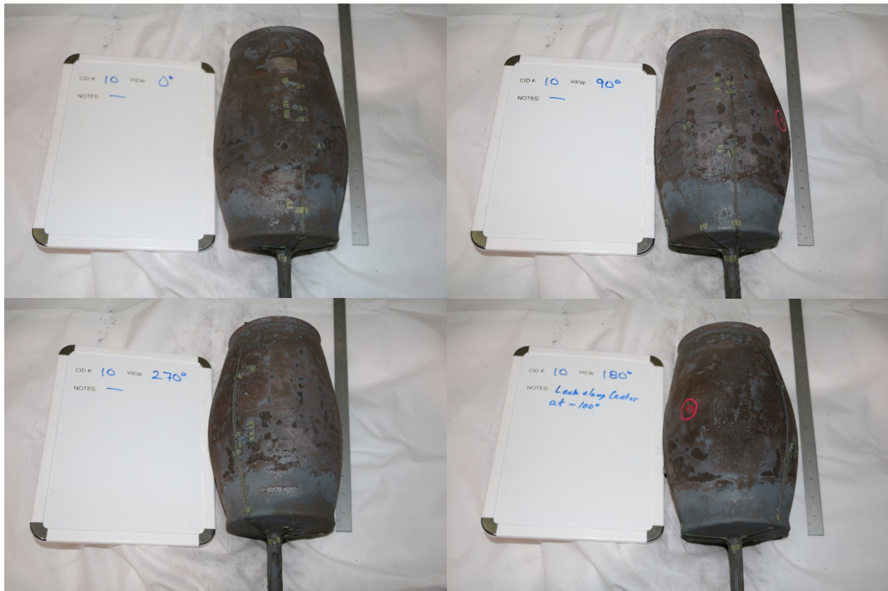
Figure 4-9. Post-test conditions of test vessel for Sequence 4. Angle positions refer to the visible portion of the vessel (see Figure 2-4). Angular positions, in clockwise direction, starting from upper left quadrant: 0°, 90°, 180°, and 270°.
