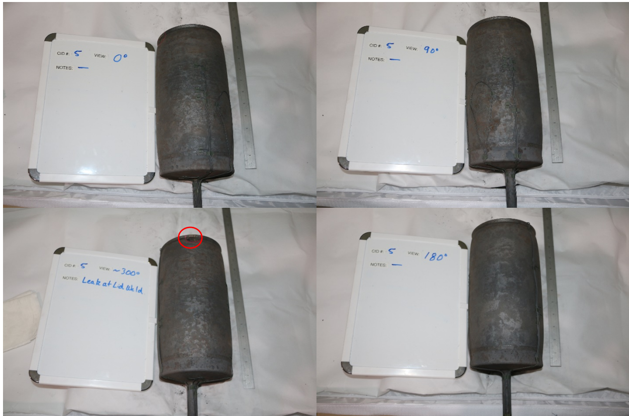
Figure 4-17. Post-test conditions of test vessel for Sequence 7. Angle positions refer to the visible portion of the vessel (see Figure 2-4). Angular positions, in clockwise direction, starting from upper left quadrant: 0°, 90°, 180°, and 300°.
