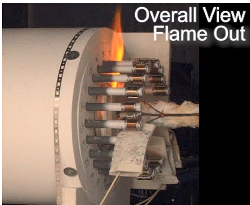
Figure 4-13. Exterior view of Sequence 5 during test, immediately after vessel was breached.
