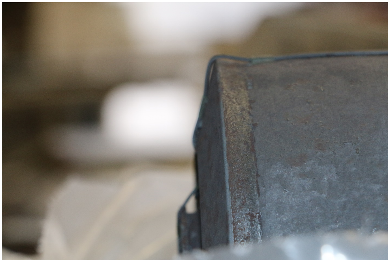
Figure 4-5. Deformation around lid region of vessel in Sequence 2.
