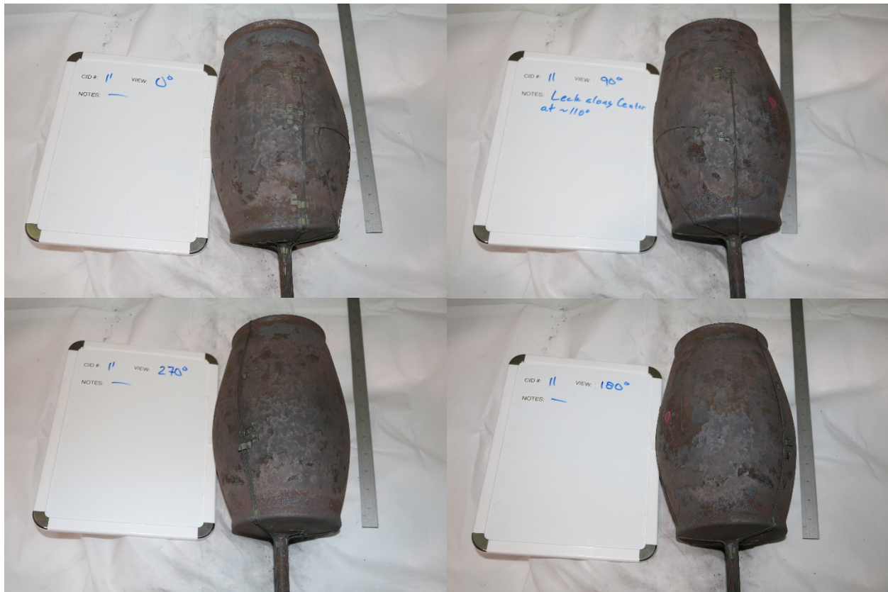
Figure 4-21. Post-test conditions of test vessel for Sequence 9. Angle positions refer to the visible portion of the vessel (see Figure 2-4). Angular positions, in clockwise direction, starting from upper left quadrant: 0°, 90°, 180°, and 270°.
