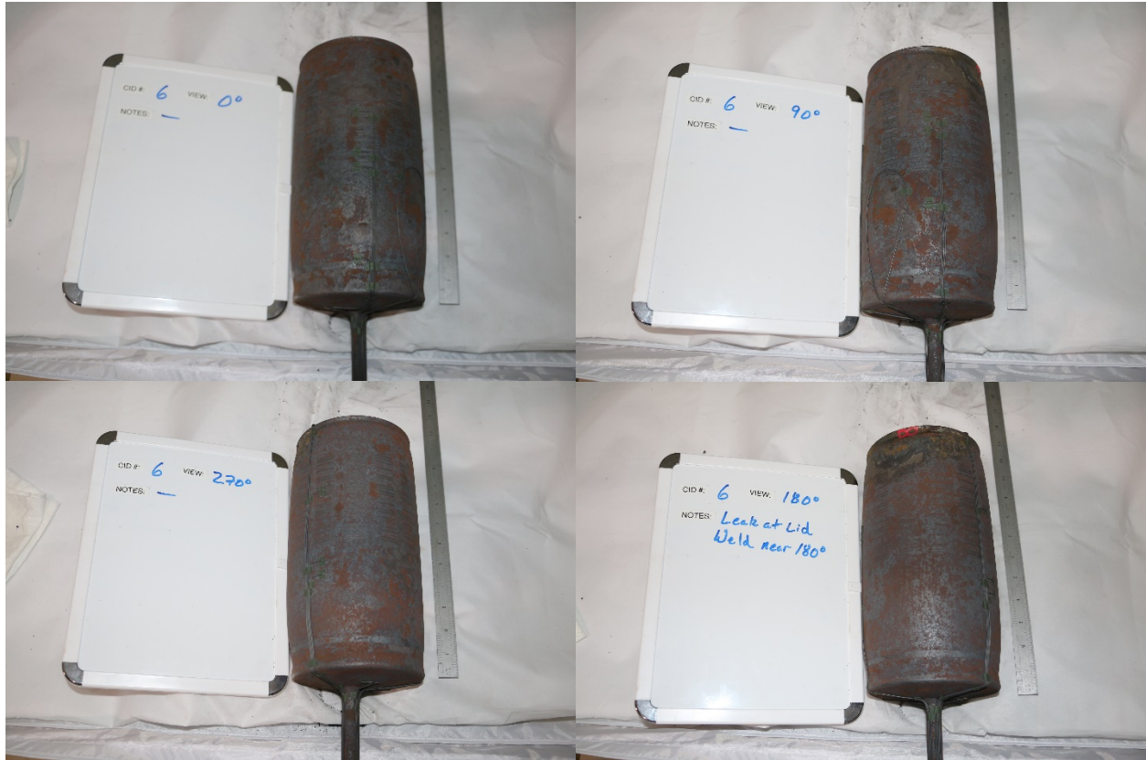
Figure 4-7. Post-test conditions of test vessel for Sequence 3. Angle positions refer to the visible portion of the vessel (see Figure 2-4). Angular positions, in clockwise direction, starting from upper left quadrant: 0°, 90°, 180°, and 270°.
