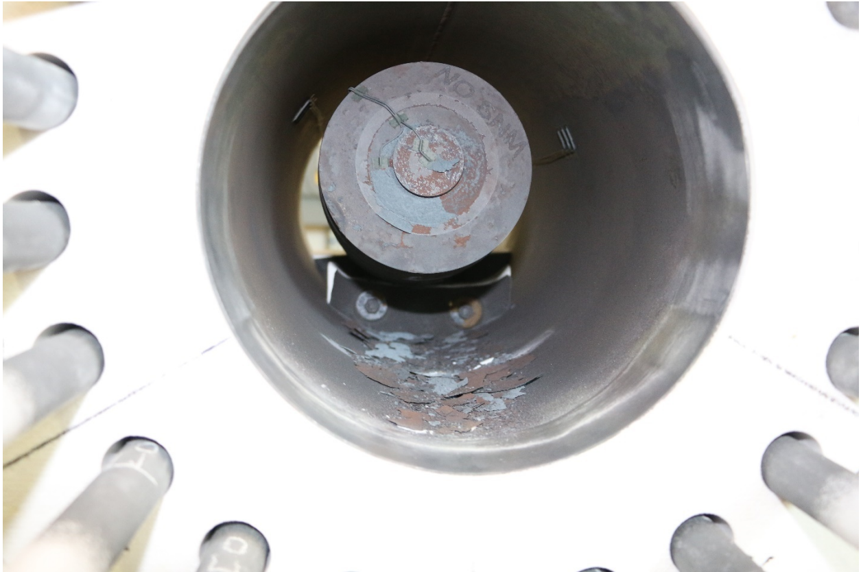
Figure 4-24. Post-test image of Sequence 10 showing debris from shroud collected at the bottom of the shroud.
