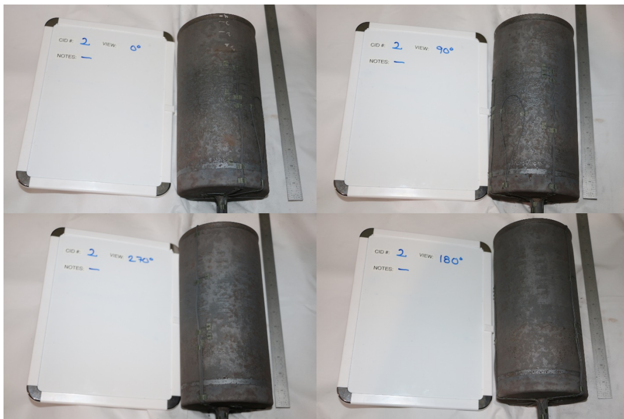
Figure 4-4. Post-test conditions of Sequence 2. Angle positions refer to the visible portion of the vessel (see Figure 2-4). Angular positions, in clockwise direction, starting from upper left quadrant: 0°, 90°, 180°, and 270°.
