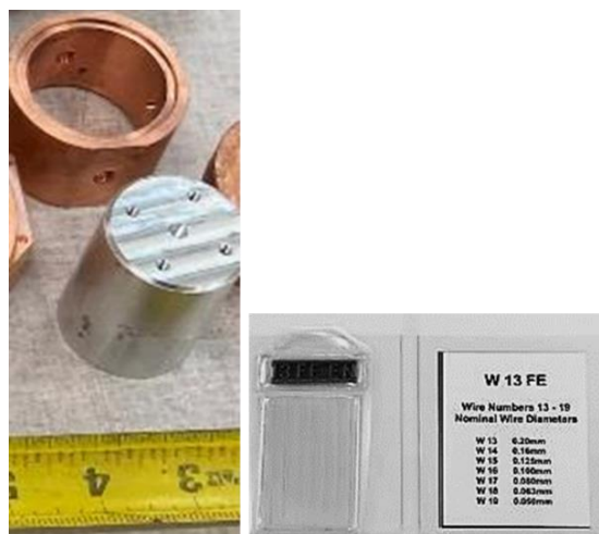
Figure 4. Phantom 1 includes an outer copper shell (6.35 mm thick) and inner aluminum cylinder (38.1 mm diameter), each with various voids. A wire gauge penetrometer was inserted in the interstitial space between the Cu and Al.
