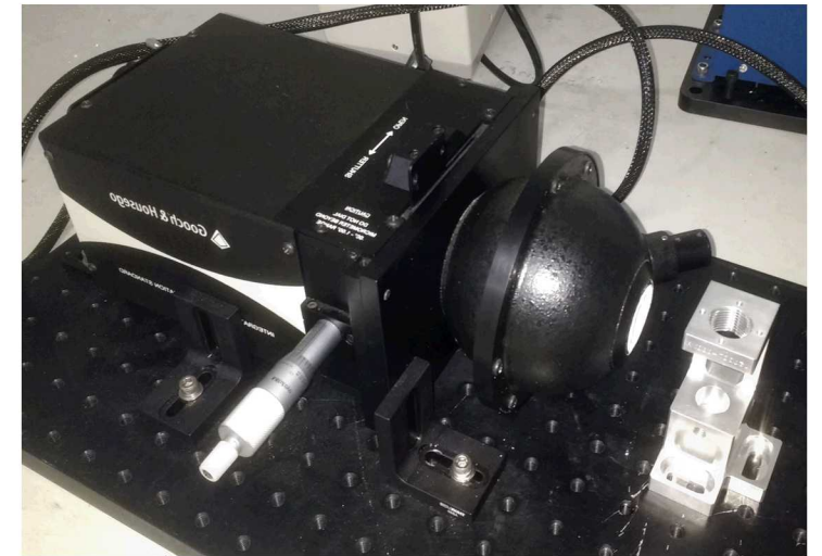
Example of cal source and integrating sphere components.
