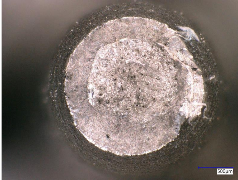
Figure A-7. Fracture Surface – R5 Parallel, 22°C, Sample 04
