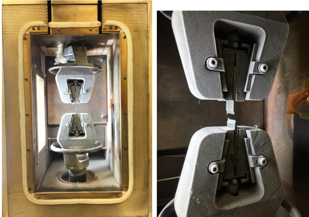
Figure 2-8. Images of the test setup for flat groove specimens are shown.
