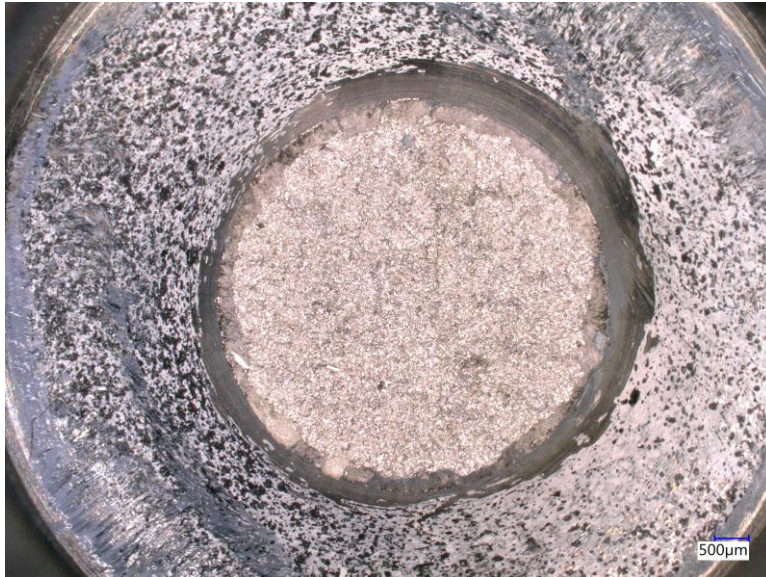
Figure A-16. Fracture Surface – 3mm, -40°C, Sample 04
