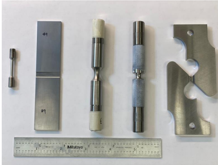
Figure 1-1. Examples of all the test specimens investigated in this study, excepting compact tension specimens, are shown. The specimens are, left to right: R5, flat-groove, 9mm notch, 3mm notch, and shear specimens.
