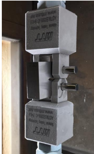
Figure 2-14. The setup for performing fracture toughness tests is shown.
