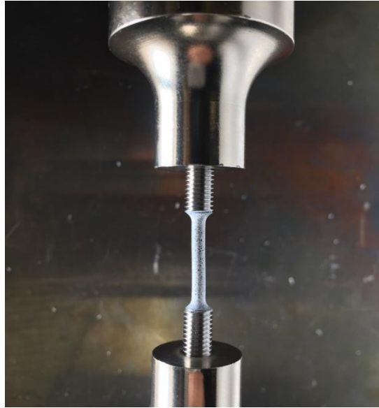
Figure 2-10. The test setup used for R5 tensile specimens is shown.
