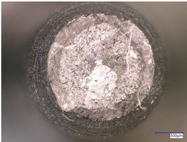
Figure A-10. Fracture Surface – R5 Radial, -40°C, Sample 12
