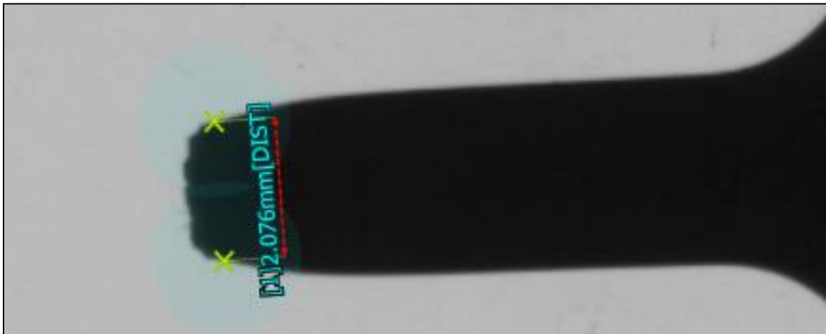
Figure 2-15. The method for measuring the diameter of fractured samples is illustrated for an R5 sample (Sample 11).
