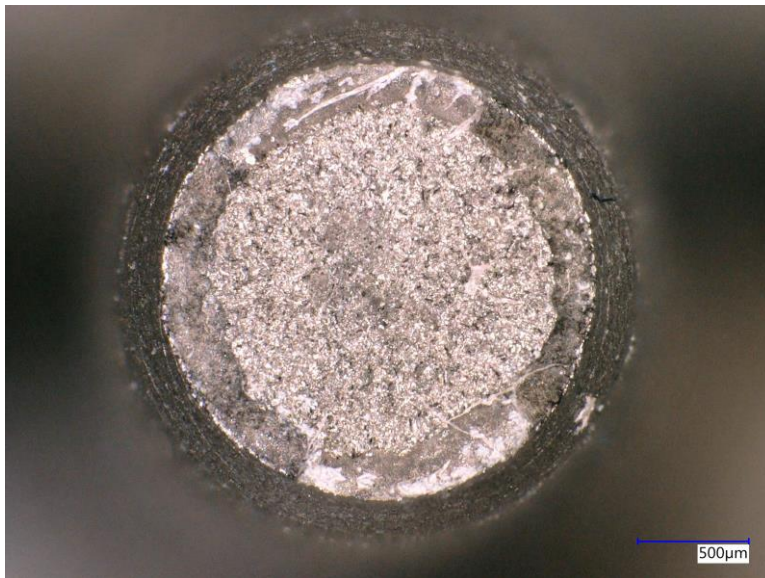
Figure A-8. Fracture Surface – R5 Parallel, -40°C, Sample 01
