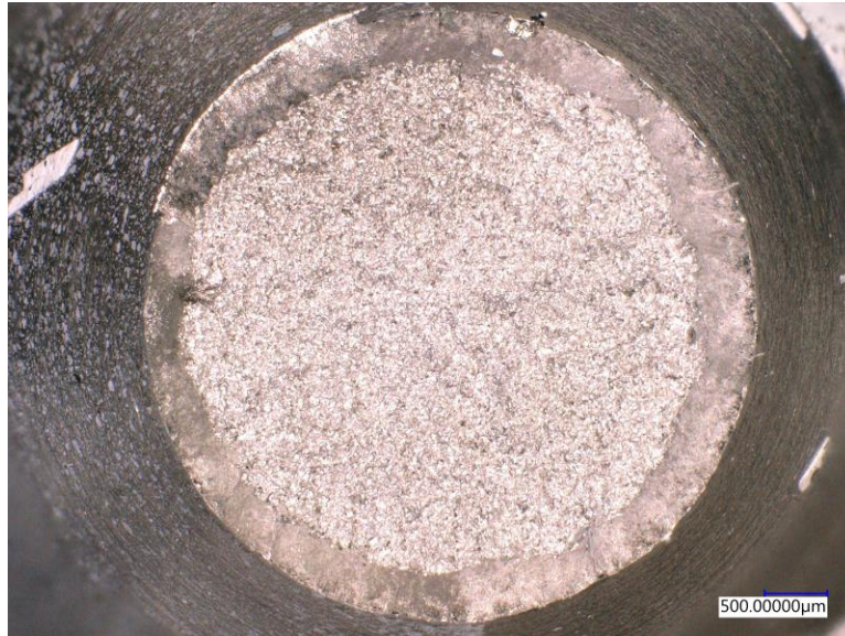
Figure A-18. Fracture Surface – 9mm, -40°C, Sample 04
