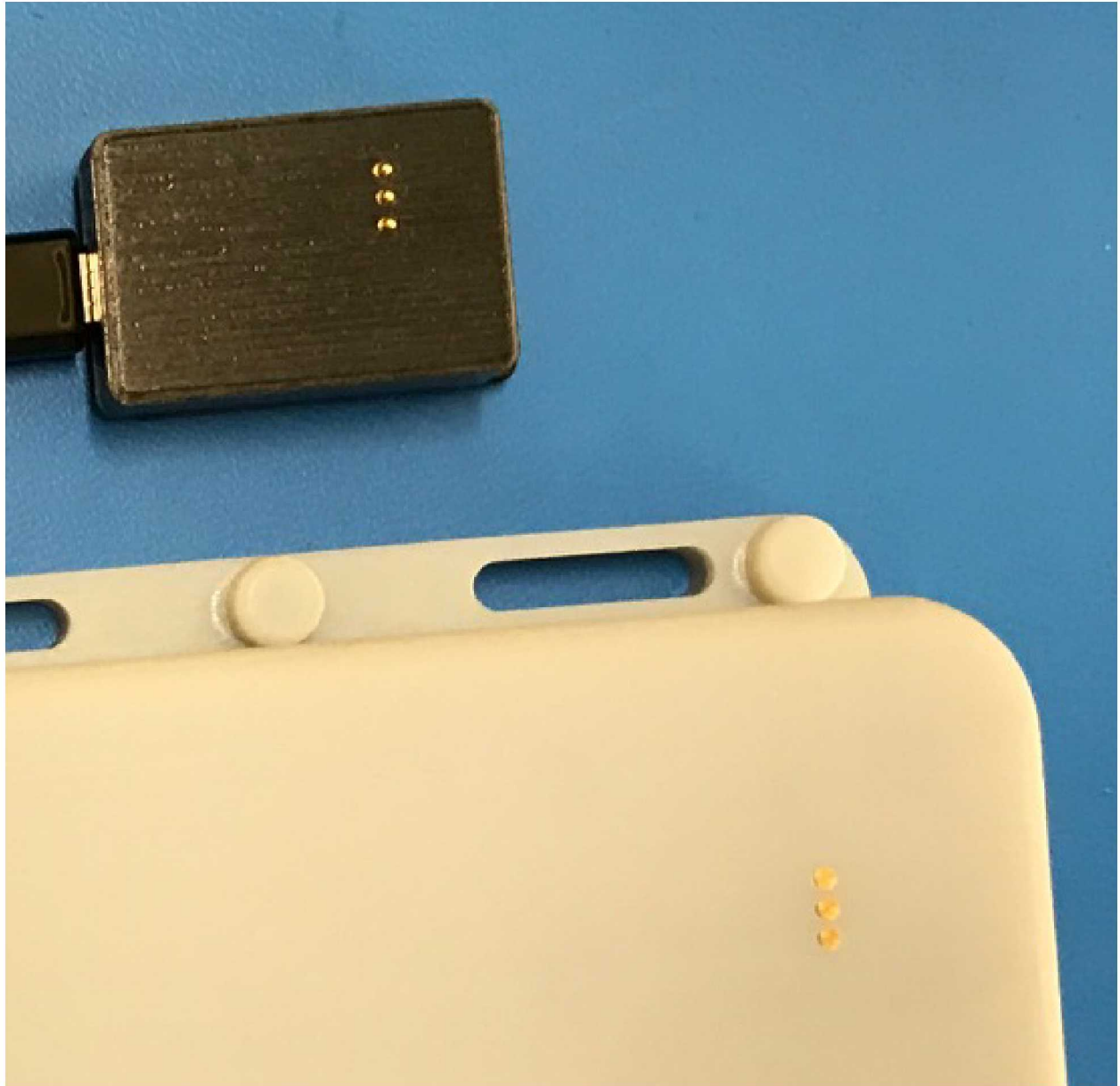
Figure 7. Static Pins Embedded in CoCIM Enclosure and Pogo Pins Embedded in Coordinator Enclosure
