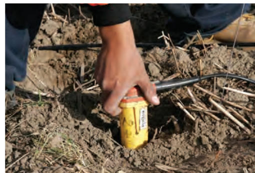
Installing sensors for seismic survey at Validation Phase Pilot Site. (Courtesy of Sarah Koenigsberg)
