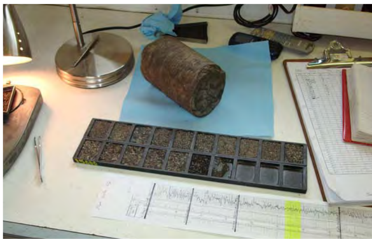
Drill core and drill chip logging from site characterization at the Mississippi Test Site. (Courtesy of Southern Company and Advanced Resources International)
