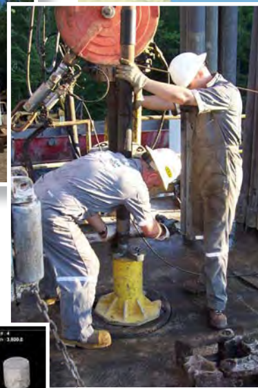
Drilling and logging work in a regional CO 2 storage exploration well.
