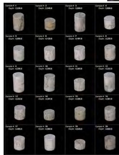
Sidewall rock core plugs sampled from a deep well.
