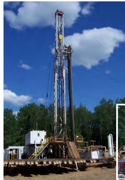
Drilling and logging work in a regional CO 2 storage exploration well.
