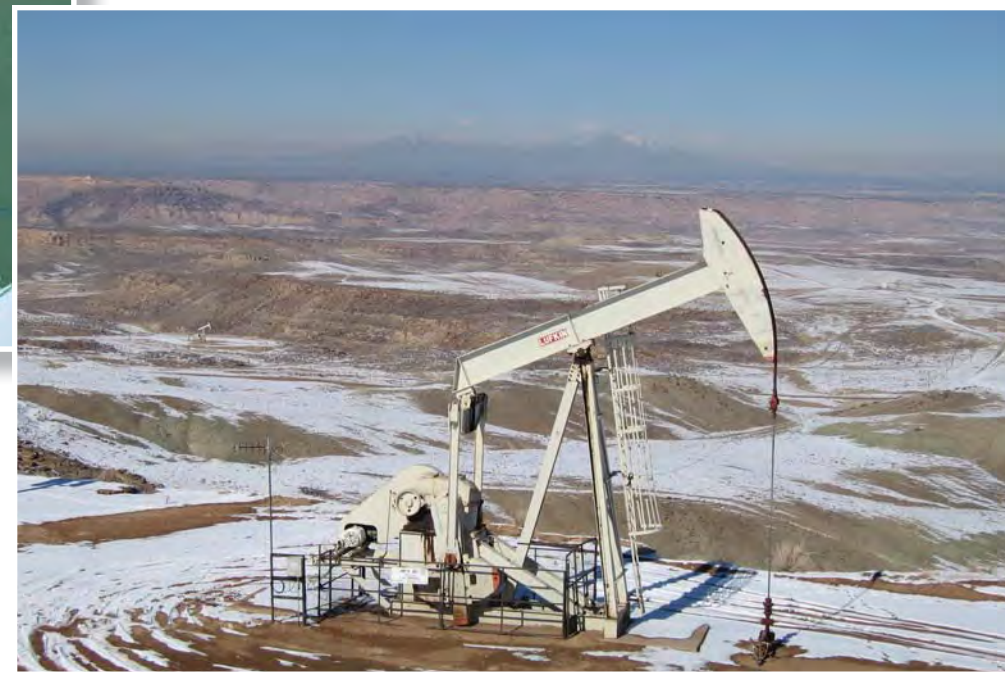
Pump jack at the Aneth Oil Field, Utah. (Courtesy of Resolute Energy)
