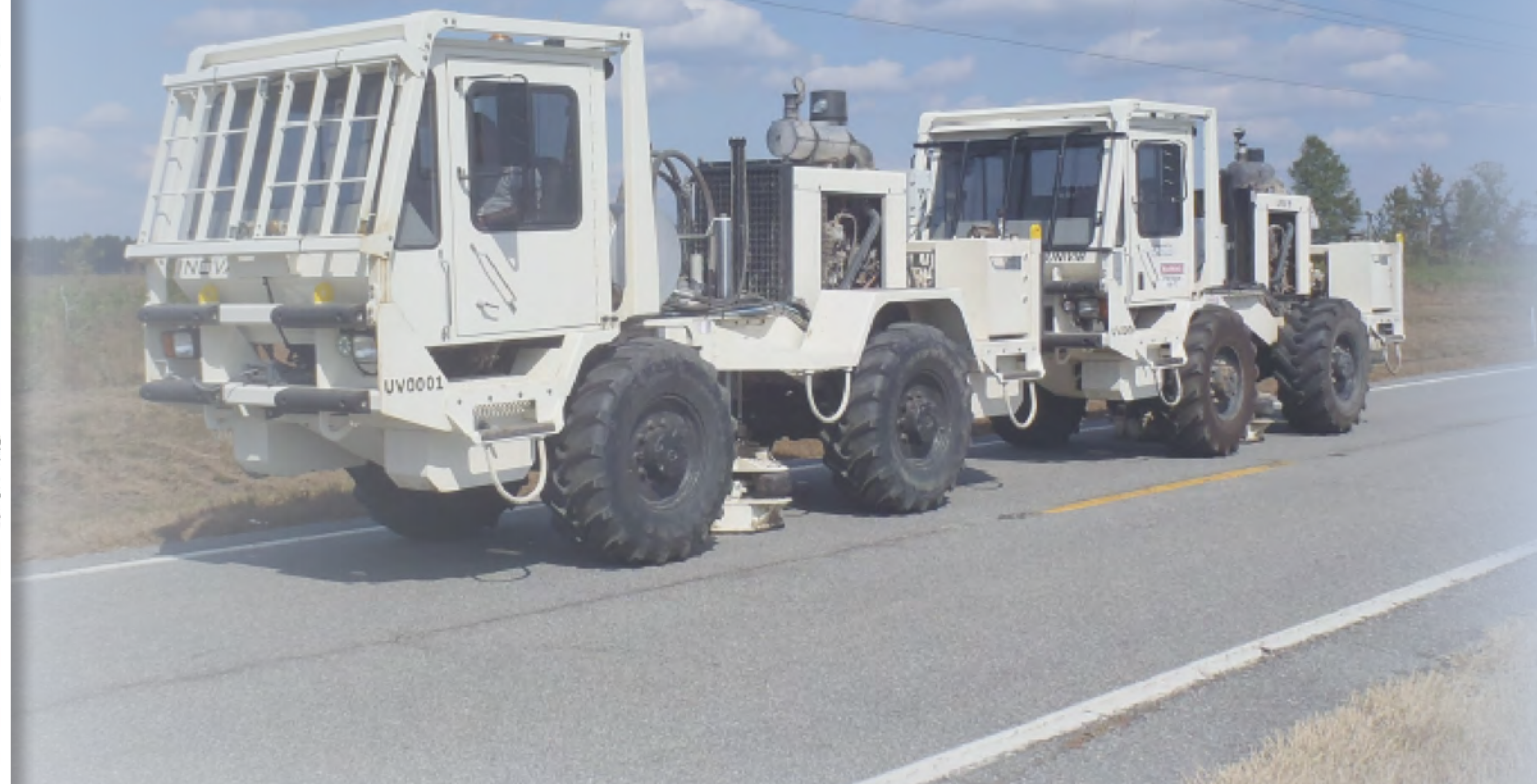
Background image: The 2-D seismic reflection acquisition by Bay Geophysical, Inc. was collected using two INOVA UNIVIB vibrator trucks along with a Wireless Seismic System, which greatly reduced acquisition time. The picture was taken along GA Line #1.
