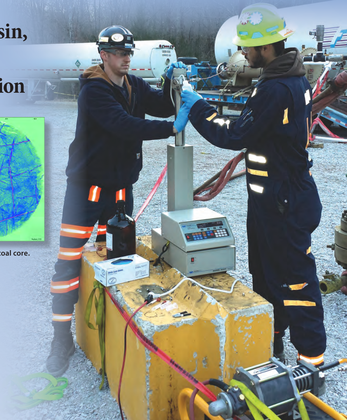
Background image: Research team injecting fluorinated tracers at the shale test site in Morgan County, Tennessee.
