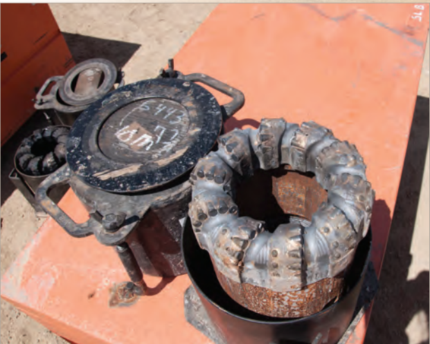
Hollow drill bits are used to extract long cylinders of rock material, known as cores. BSCSP acquired approximately 450 feet of core from both wells.
