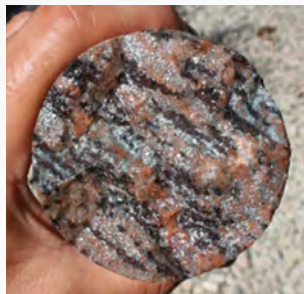
Core recovered from crystalline basement (contact at 1,712 feet).
