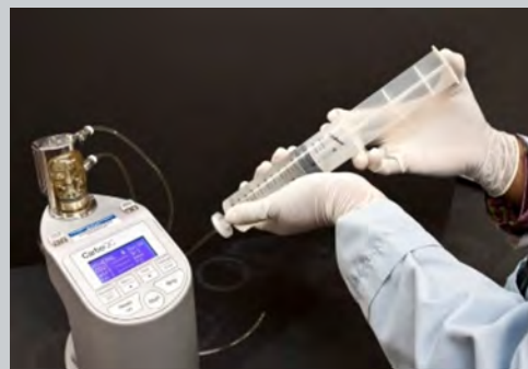
NETL researchers in conjunction with collaborators at West Virginia University pioneered the use of a CarboQC carbonation meter used in the beverage industry (manufactured by Anton Paar) for the direct measurement of CO 2 in waters in the field setting.
