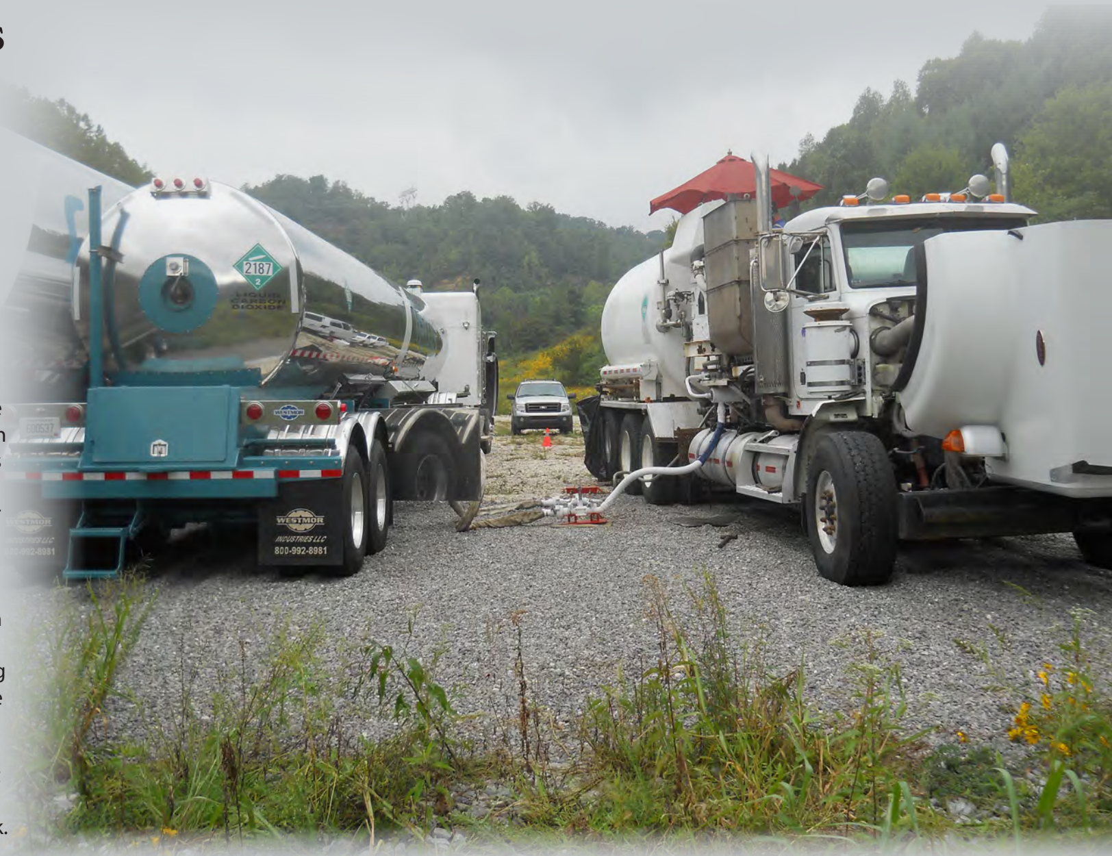
Background image: Onsite CO 2 facilities with storage vessel (far left), over-the-road transport with transfer pump (left), and CO 2 connected to a nitrogen fracture stimulation truck (right) where the CO 2 was vaporized, heated to 100 °F, pressurized, and pumped to the SS-#1 test well.
