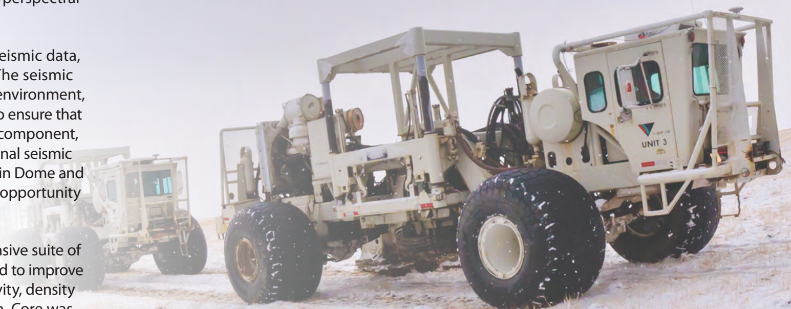
Background image: Vibroseis "thumper" trucks conduct seismic surveys of the underground geophysical environment.
