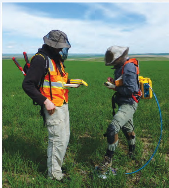
Field crew use a portable soil fluxmeter to measure the amount of CO 2 within the soil located near the proposed injection well site.
