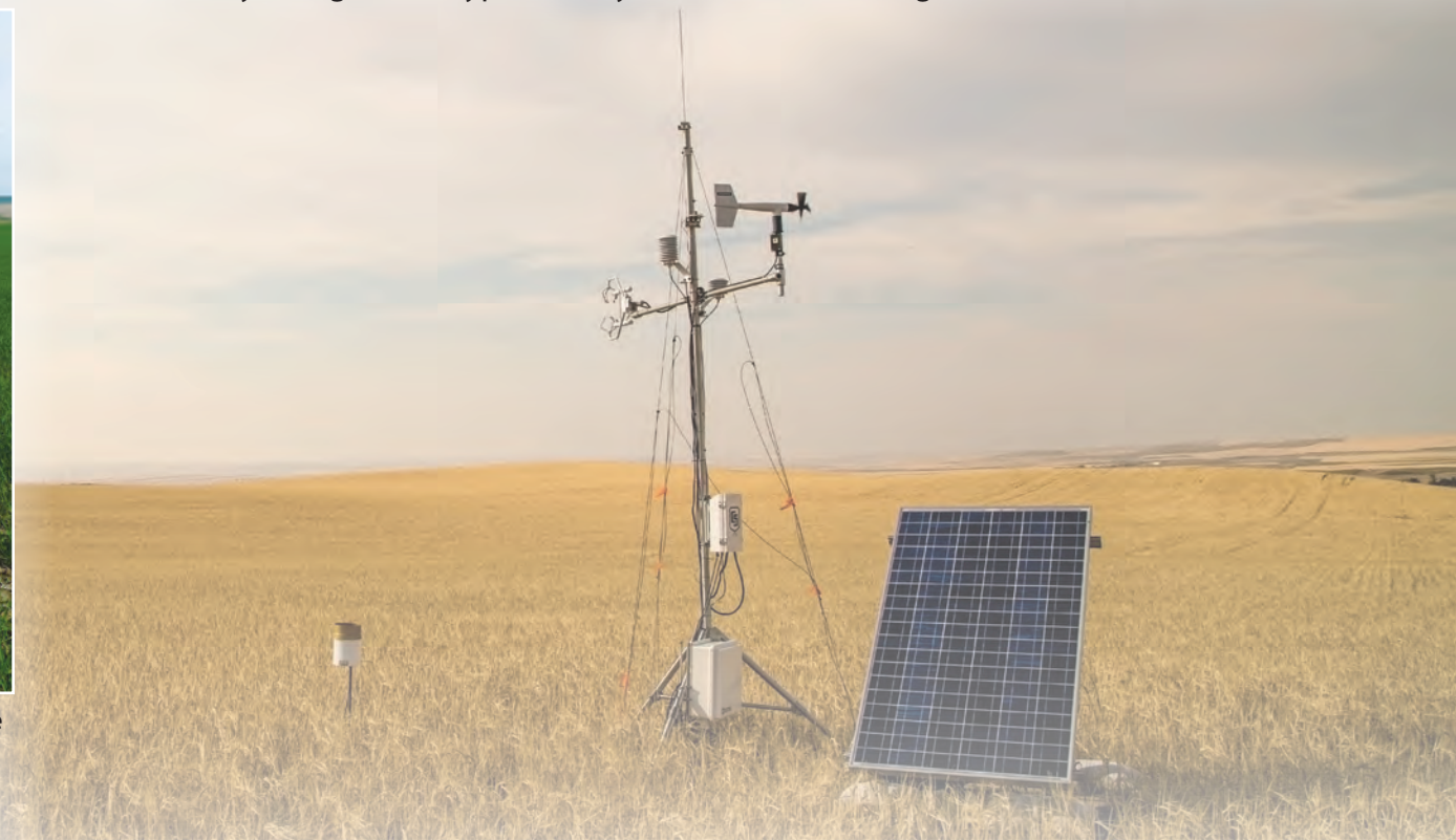
Background image: An eddy covariance tower and a weather station were installed in the project area to monitor net CO 2 flux and meteorological variables.
