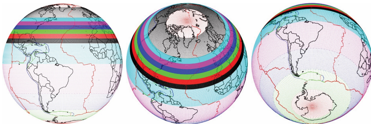
Figure 1. Sampling strategy using latitude bands. In this case, the Earth is broken into 13 latitude bands with high resolution bands in the northern hemisphere across North America and Eurasia, and low- resolution bands at the poles. Regular grids with LLNL-Earth3D user defined \Delta Lat and \Delta Lon spacings are constructed and output to separate files to be read into SPEC-FEM3D_GLOBE for computing finite element properties.
