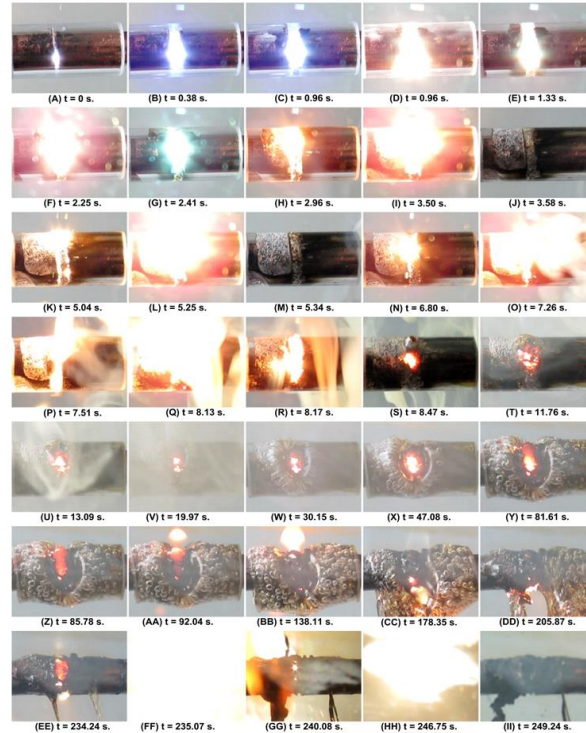
Figure A2–5. Polycarbonat tube with no hole example test. Possibly fire ignition at 7.26 s, but no sustained external flame until after 92.04 s.
