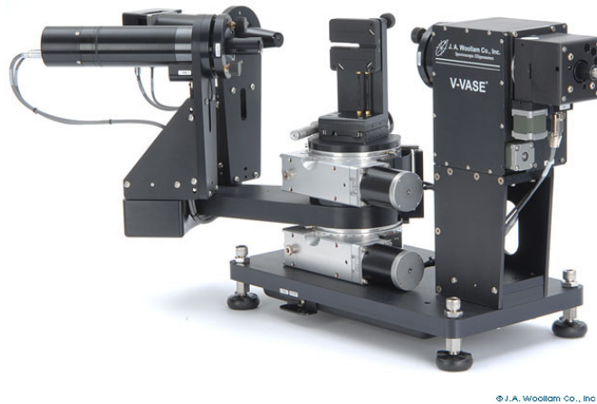
Figure 3. Benchtop, variable angle, spectroscopic ellipsometer (Woollam, Inc.) used in this study of optical constants for laser color marked samples. Image from Woollam website.
