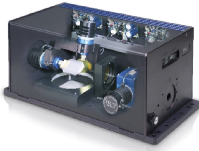
Figure 16. Nutfield Technology's 3-Axis Contour designed for laser color marking large surface area and shaped (nonplanar solids). Enclosure is roughly 30 x 30 x 70 cm. https://www.nutfieldtech.com/3xb-3-axis-scan-head/
