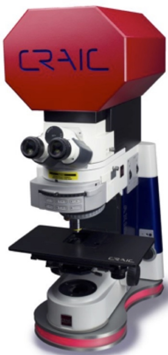
Figure 2. Benchtop microspectrophotometer (CRAIC) used for the evaluation of color islands on laser marked, bulk stainless steel 304L samples. Image from CRAIC website.
