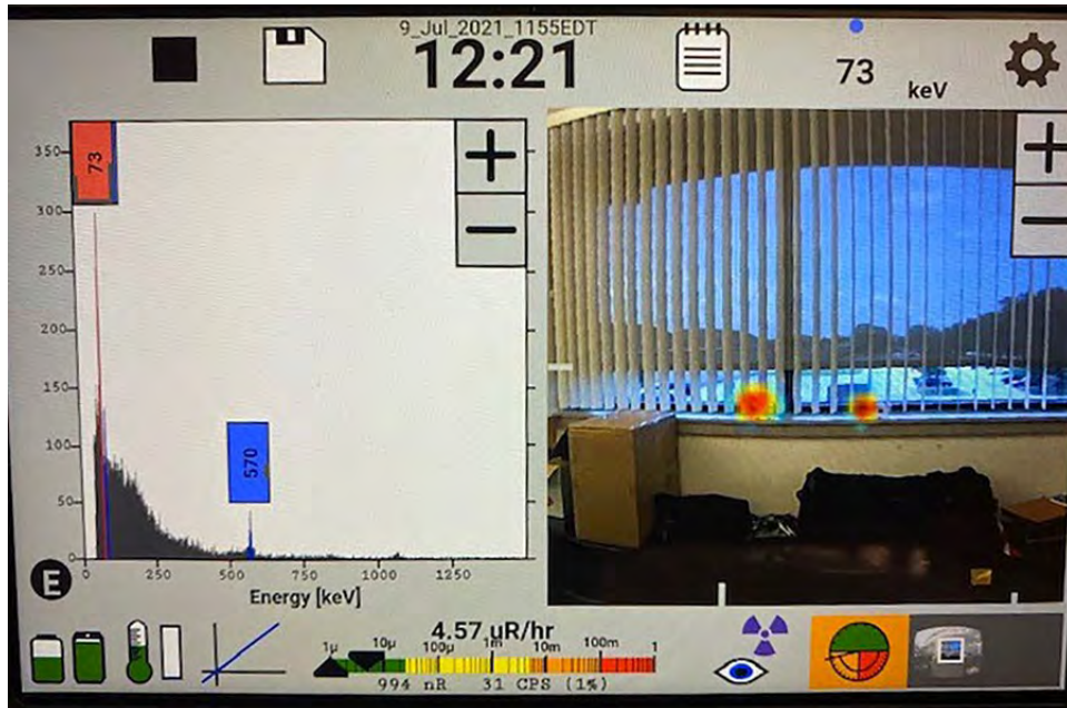
Figure 4. Optical and radiation images of two button sources (each of ^{207}\text{Bi} isotope) placed 0.58 m apart. The sources were imaged with enough clarity to be distinguished from a perpendicular distance of 2.4 m. The time taken to image was 12 minutes 21 seconds. Compton rings of colored bands started to show long before a good quality image was obtained.
