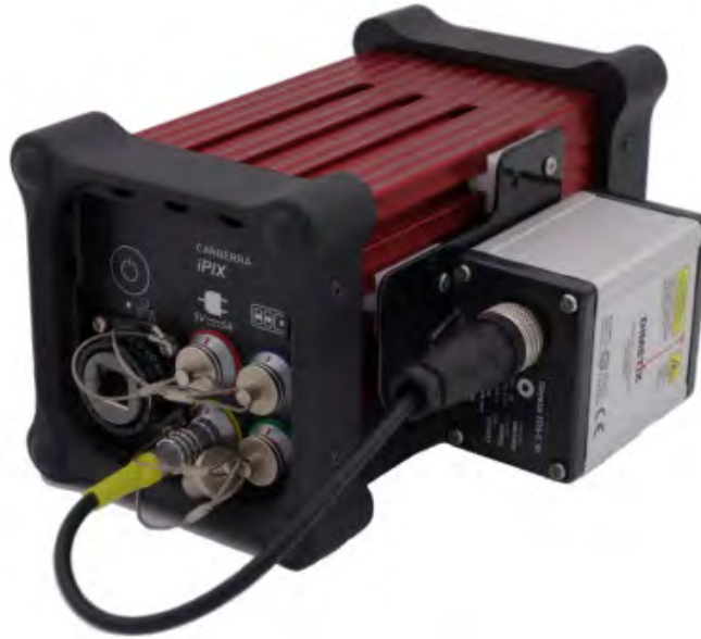
Figure 2. iPIX gamma imager is a lightweight camera that uses pixelated CZT crystal with MURA rank 7 and rank 13 coded apertures.
