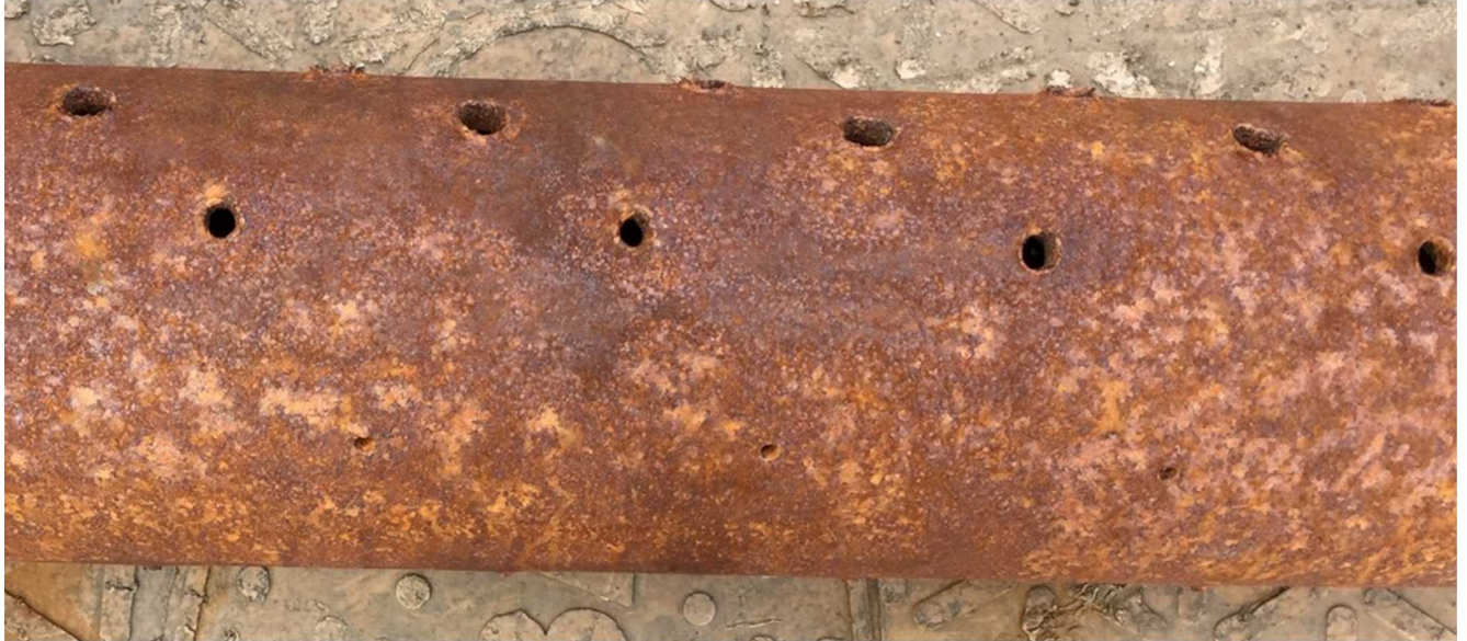
Figure 4 Perforated casing with entry hole diameter variance due to gun decentralization. From top of photo wrapping towards the bottom, this shows holes from rows 6, 3, 8, and 5 (see Figure 5).
