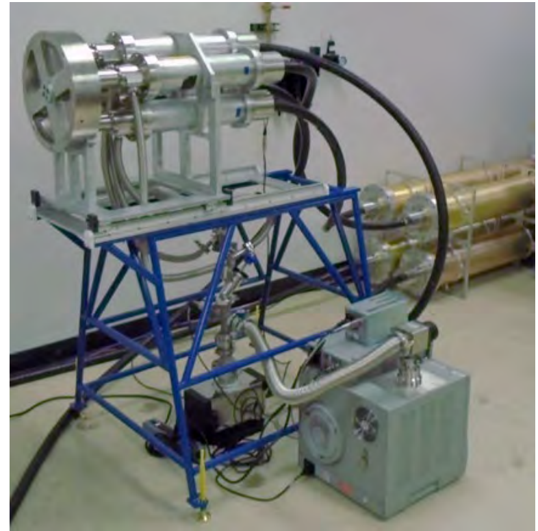
A modern four-pulse soft x-ray head with Supersaver Marx banks in background
