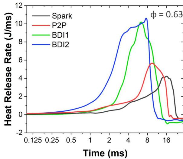
Since laminar-to-turbulent kernel period has the most variability, shorter periods are expected to benefit engine combustion stability
