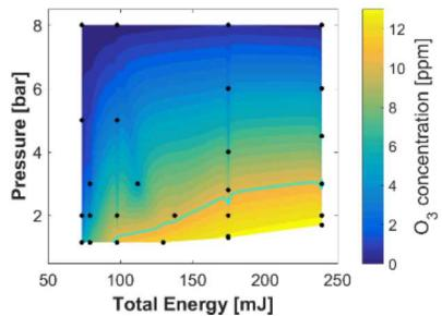
**NRPD BDI is effective at generating sufficient  $O_3$  quantities via early-cycle discharges**
