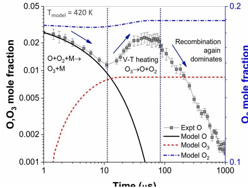
Low global O formation and potential  $O_3$  destruction from V-T heating makes this pathway unviable
