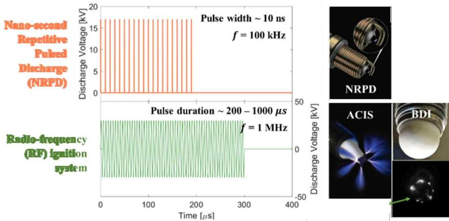
Fundamental NRPD research is focused on corona, glow, arc, and surface discharge ignition
