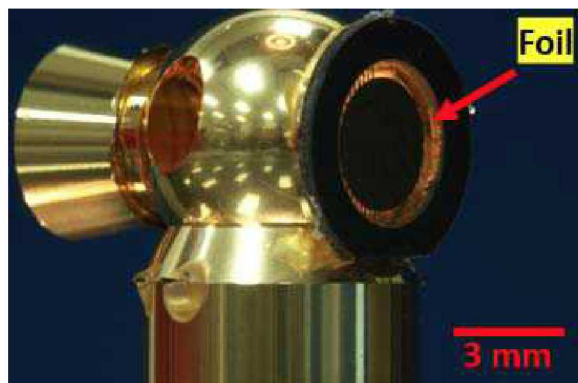
Sample on hohlraum w/ Be tamper attached
