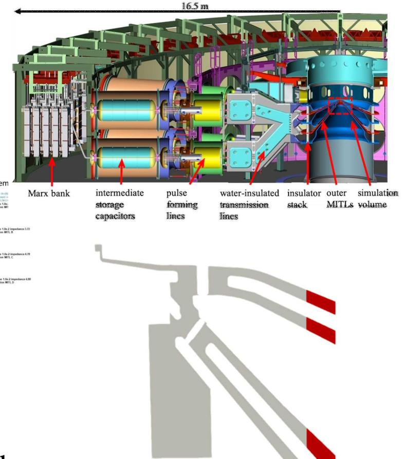
MITL flow is traditionally modelled using particle-in-cell techniques, which can be costly due to need to resolve Debye length. Relativistic fluid models provide an alternative that offer reduced computational cost.
