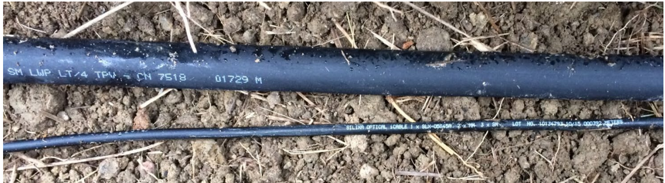
Figure 5. Two co-located fiber-optic cables from the Aquistore site, showing the helical wound cable (top) and straight tactical cable (bottom).
