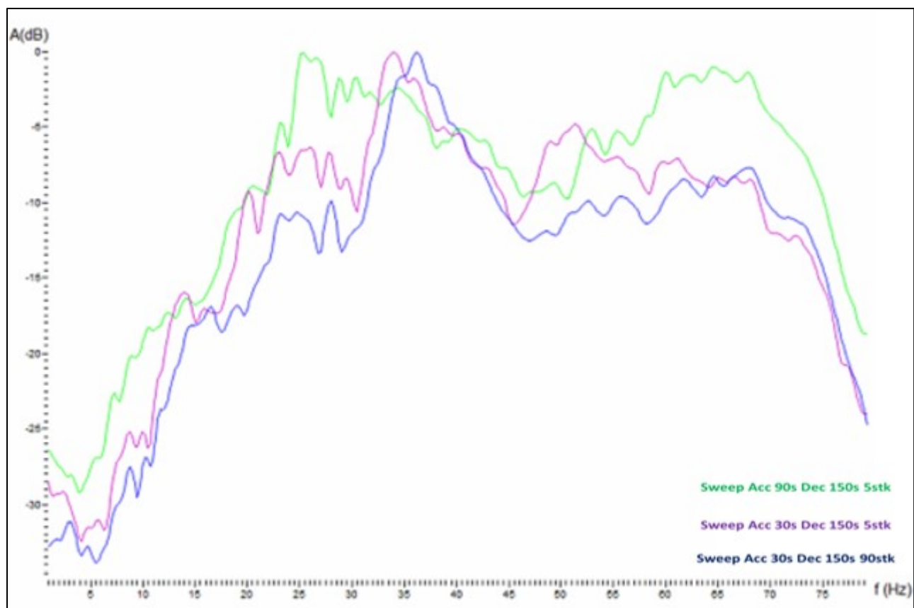
Figure 46. Frequency spectrum comparison of the new sweep parameters vs. historic using SOV#4.
