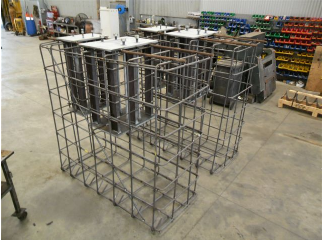
Figure 7. Rebar cage with I-beam reinforced mounting plates. Each rebar cage has a mount for both a small 4 T-f SOV and a 10 T-f SOV (Otway Project).
