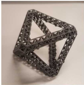
Figure: Hierarchical multiscale structure of octahedral (second-order). Printed in Georgia Tech Invention Studio.
