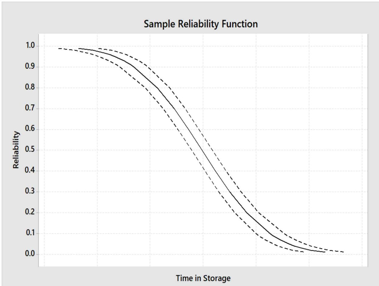
Reliability function based on degradation measure effect on performance
